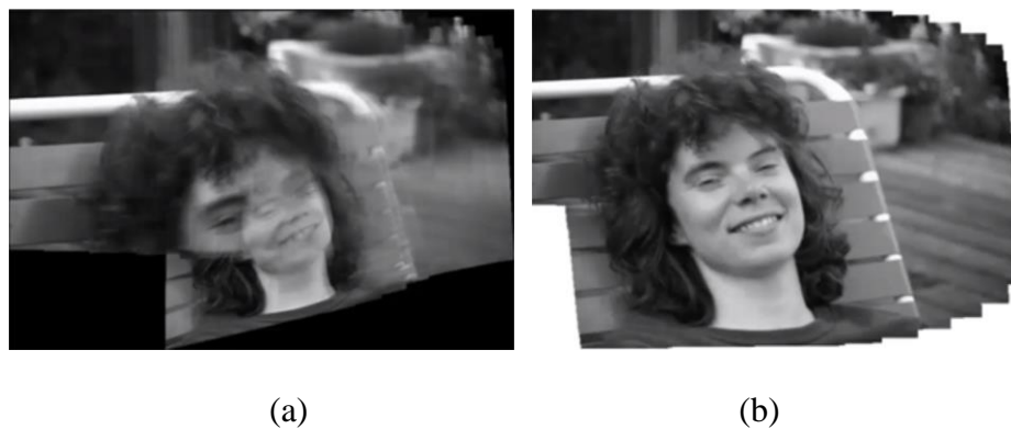
Fig. 1.2. Comparison between affine mosaic and projective mosaic. (a) Affine mosaic. (b) Projective mosaic [32].
