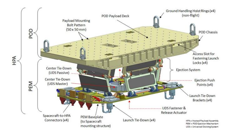
Figure 4: Standard Hosted Payload Assembly (HPA) in Deployed Configuration Patent Pending (PCT/CA2015/050451)
