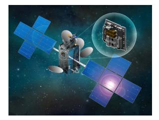
Figure 2: SSL Satellite Locations Frequently Available for POD RideShare – Mid-Panel on East/West Faces (Extended Size)
