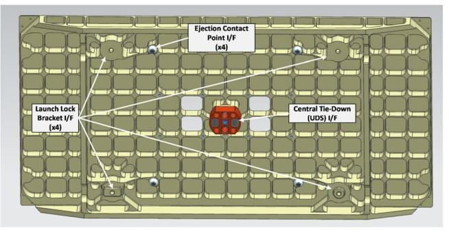
Figure 5: Standard POD Chassis (Underside) to PEM Interfaces
