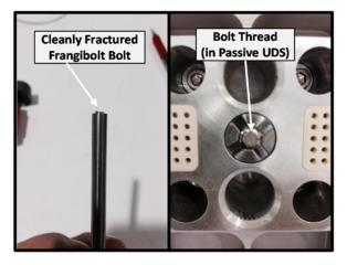
Figure 7: UDS Fastener Release Test – Severed Fastener
