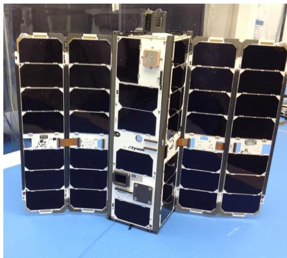
Figure 1 - CPOD Vehicle Configuration
