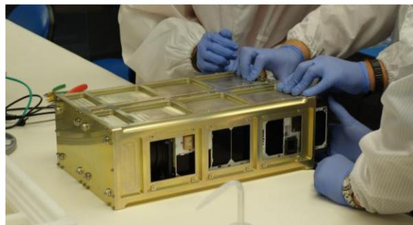
**Figure 10 - CPOD Engineering Unit Integrated in Tyvak 6U Deployer for Qualification Testing**
