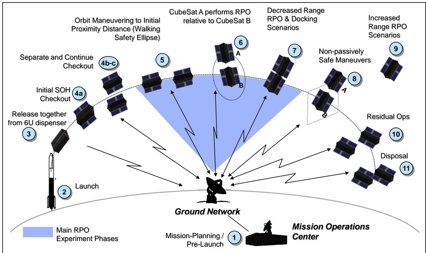
Figure 2 - CPOD Concept of Operations
