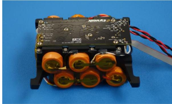
**Figure 5 - 60Whr Battery Pack in a 3S2P Configuration with Battery Heaters**
