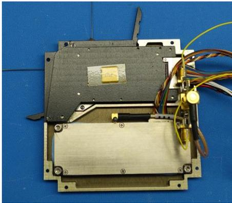
**Figure 4 - UHF Transceiver with Deployable Antenna and S-Band Transmitter**
