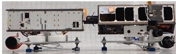
**Figure 11 - Air Table Testing**
