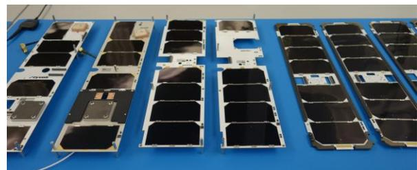
**Figure 6 - Fixed and Deployable Solar Panels with PPTs, Antennas, and Umbilical Interfaces**
