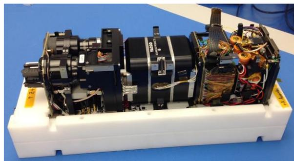
**Figure 8 - Internals of CPOD showing 1U of RPOD Payload (Left), 1U of Propulsion (Middle), and 1U of Avionics (Right)**
