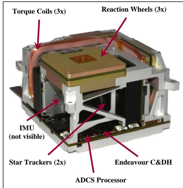
**Figure 3 - Inertial Reference Module (IRM)**
