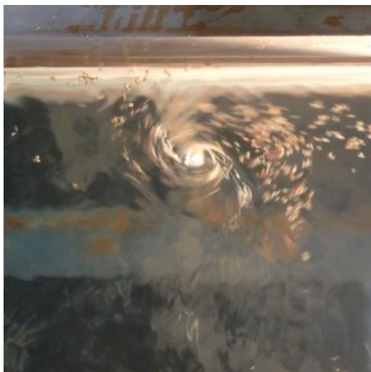
Figure 31. Type 5 vortex at Q1 in model B.
