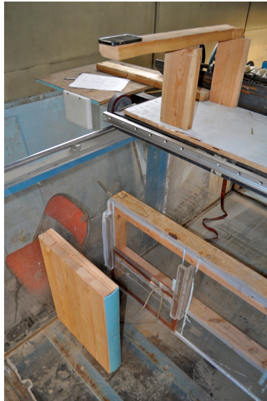
Figure 14. Camera mount for overhead video recording installed in model B.
