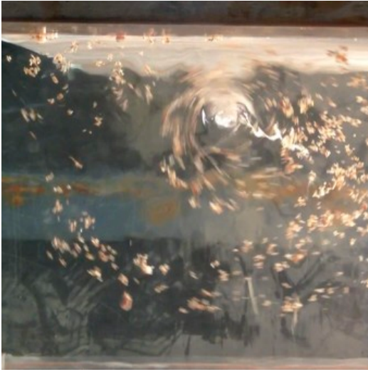
Figure 35. Type 5 vortex at Q2 in model B.
