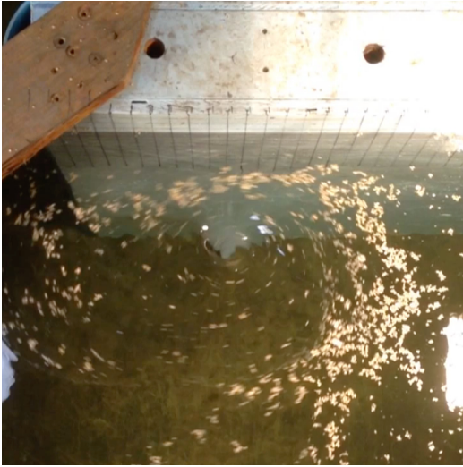
Figure 34. Type 5 vortex at Q2 in model A.
