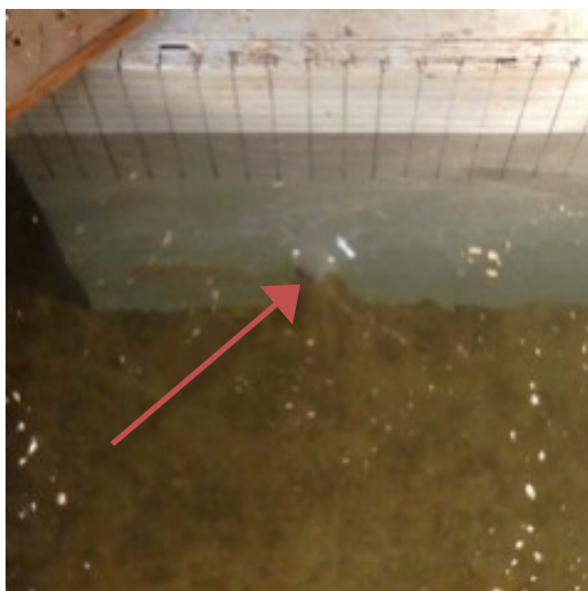
Figure 38. Type 4 vortex at Q3 in model A.
