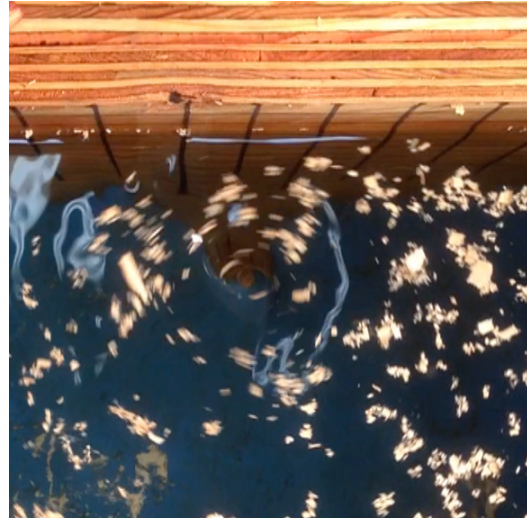
Figure 36. Type 5 vortex at Q2 in model C.
