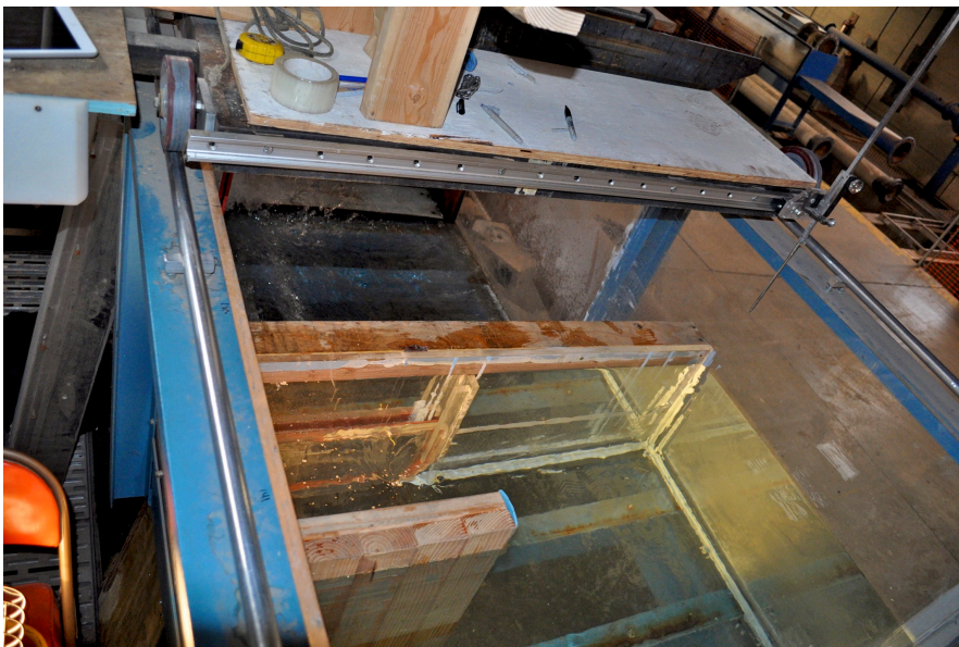
Figure 10. Model B experiment model installed in 4-foot flume.
