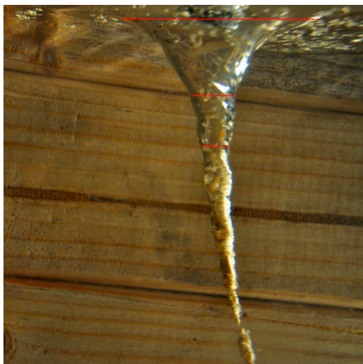
Figure 23. Type 5 vortex at Q2 in model B.
