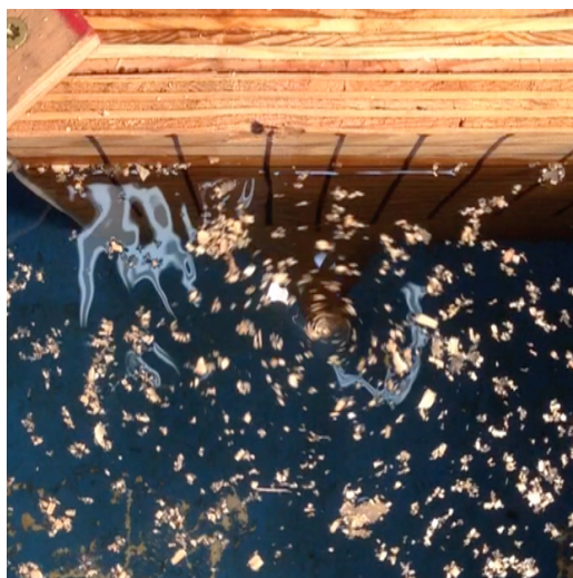
Figure 40. Type 4 vortex at Q3 in model C.
