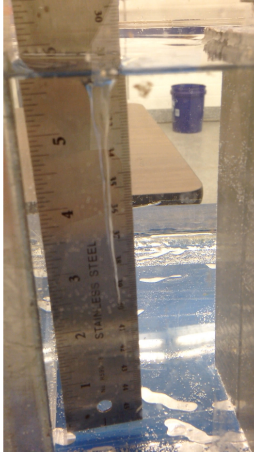
Figure 51. Type 6 full air core vortex forming with a modified approach in model D.
