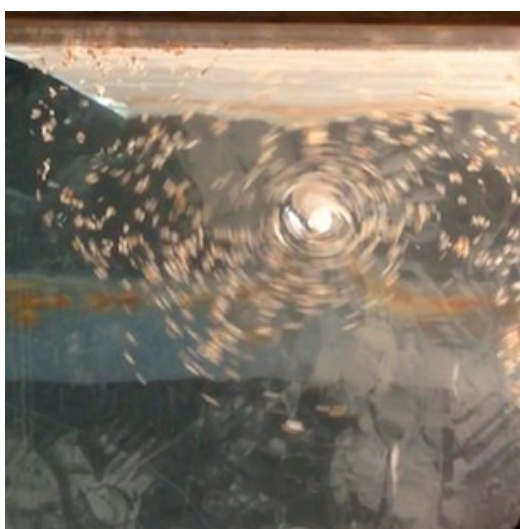
Figure 39. Type 4 vortex at Q3 in model B.
