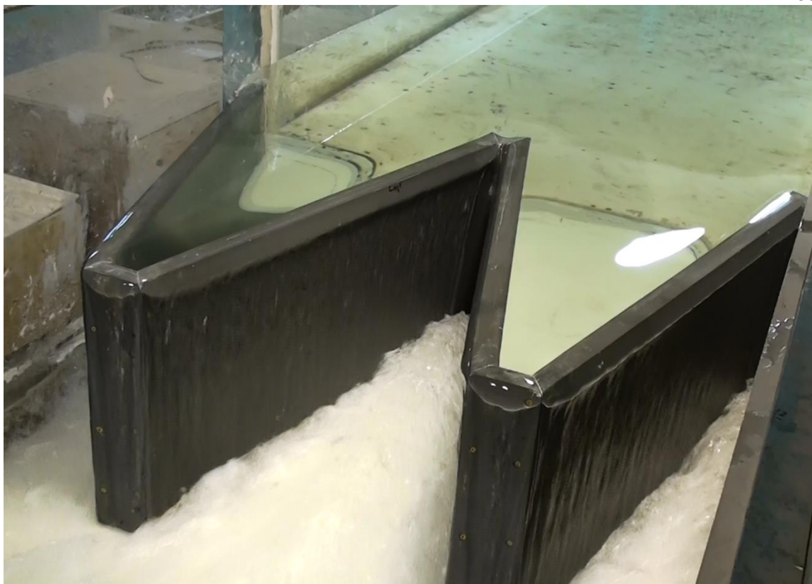
Fig. A-19. \alpha = 15^\circ , QR , A=1t_w , normal orientation, H_T/P = 0.1 , P=18 in, photograph
