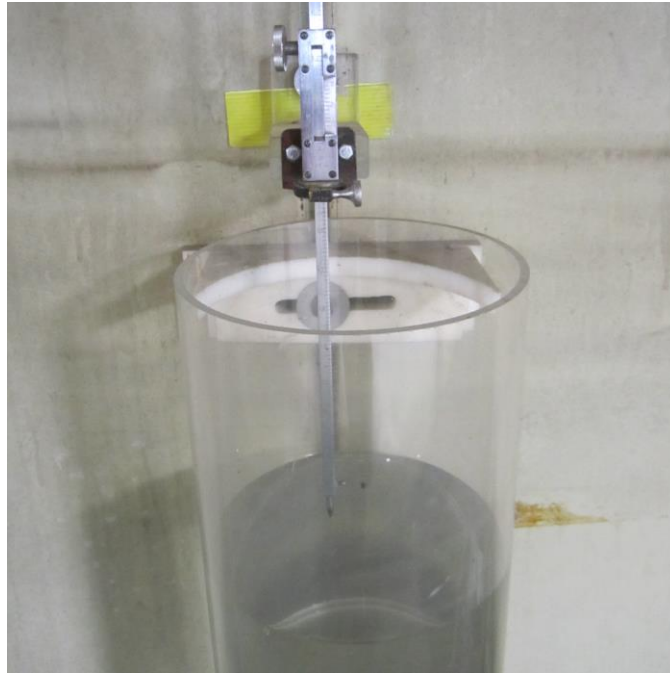
Fig. 11. Stilling basin with point gage
