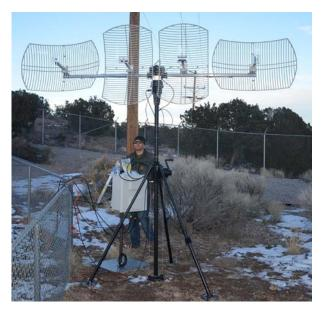
Figure 4: Prometheus High Band Antenna with Outdoor RF Box
