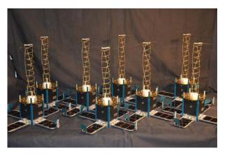
Figure 1: Eight Prometheus Flight Units (shown in post-deploy configuration)
