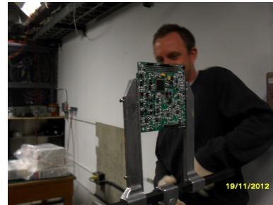
Figure 6: The complete electronics platform being prepared for exposure to proton flux at the Crocker Nuclear Laboratory, UC Davis.
