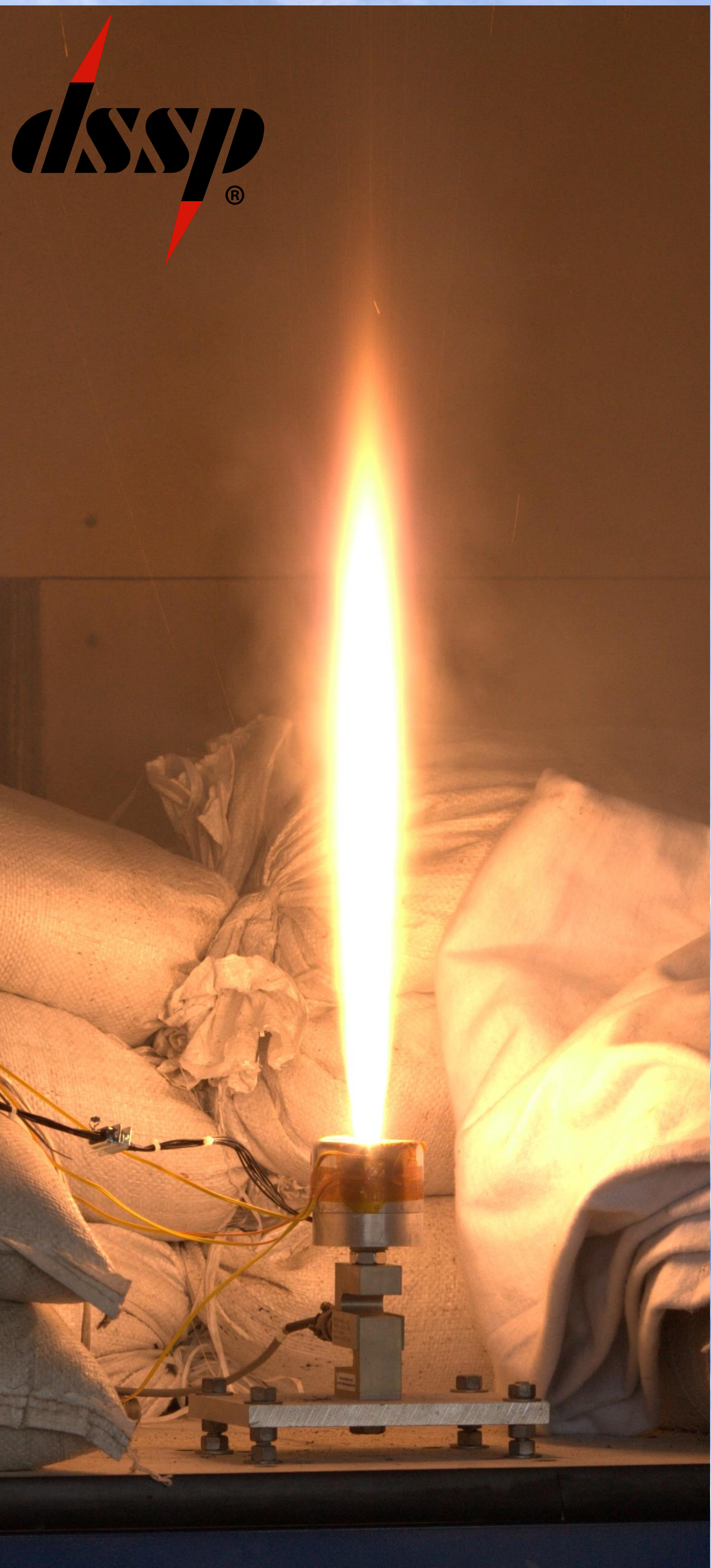
Firing of a CDM-1 development motor in the DSSP test cell
