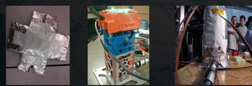
Figure 6 Cryogel Z blanket (left). The CubeSat without the insulation (center), and with the insulation (right).
