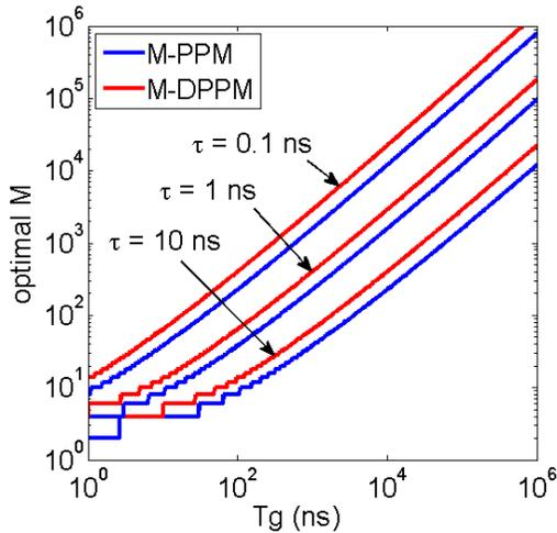
**Figure 1: Slot number,  $M$ , that maximizes the data rate for  $M$ -slot Differential Pulse Position Modulation (M-DPPM) and Pulse Position Modulation (M-PPM) schemes for a given  $\tau$  and  $T_g$ .**
