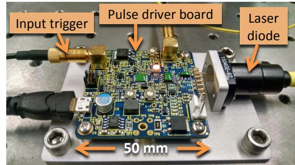
**Figure 8: Picosecond laser driver and 1550 nm fiber seed laser**
