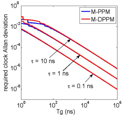
**Figure 3: Required clock Allan Deviation for the M-DPPM and M-PPM schemes for a given  $\tau$  and  $T_g$ .**
