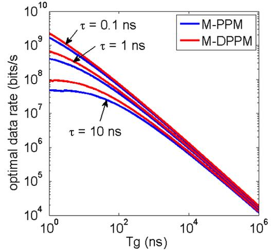
**Figure 2: Optimal data rates for the M-DPPM and M-PPM schemes for a given  $\tau$  and  $T_g$ .**
