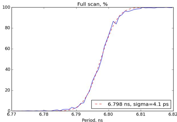
**Figure 7: Fraction of ones at the DLL arbiter close to the transition**
