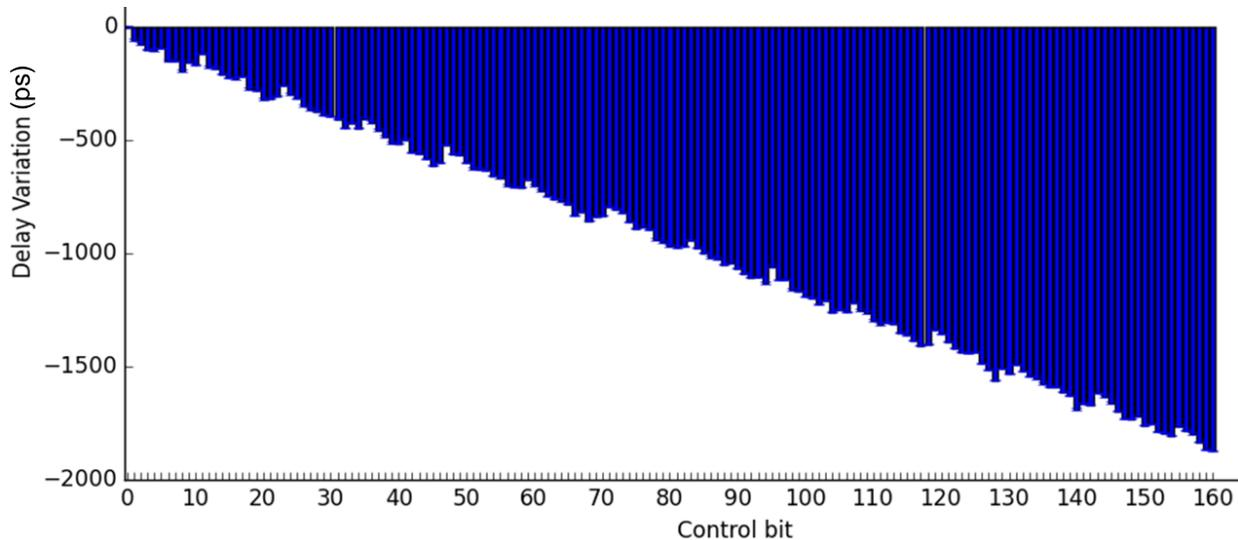
**Figure 5: Delay chain propagation delay as a function of control input**
