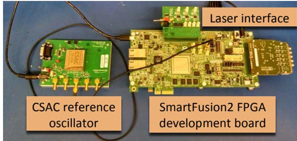
**Figure 9: Software-Defined Pulse Modulator consisting of the SmartFusion2 FPGA, CSAC and laser driver interface board**
