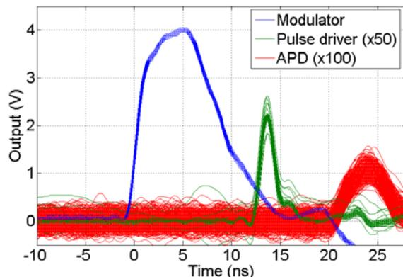
**Figure 12: A sequence of 500 overlaid pulses produced by the modulator (blue), pulse laser driver (green), and recorded by the APD (red).**
