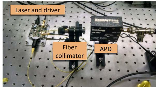
**Figure 11: 1550 nm diode laser driver, fiber collimator and avalanche photodetector (APD)**
