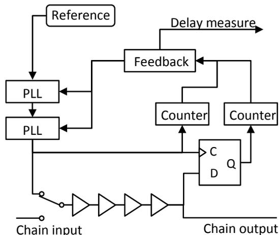
**Figure 6: Delay Locked Loop block diagram**
