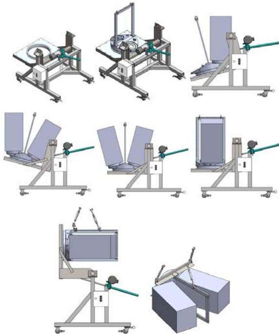
**Figure 19: Payload and DPA to SHERPA Integration Steps (Image Credit: LoadPath)**
