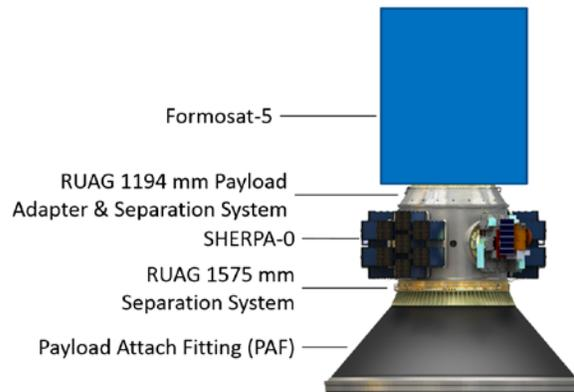
**Figure 16: Integrated Payload Stack**
