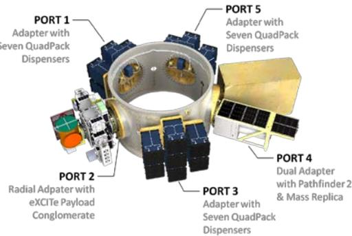
**Figure 21: SHERPA Payload Arrangement**
