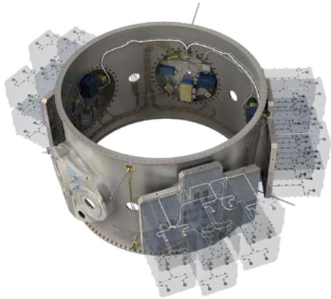
**Figure 6: Illustration of SHERPA Flight Harness**
