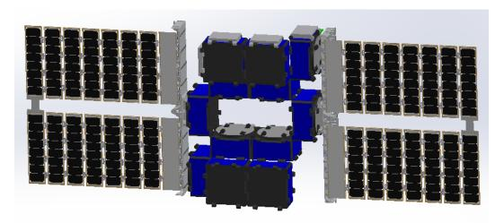
Exhibit 2: Payload Testbed-2 – A PAC of twelve aggregated HISats shown with two deployed solar arrays
