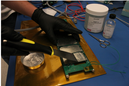
Figure 3: Applying silicon epoxy to PCB with putty knife.
