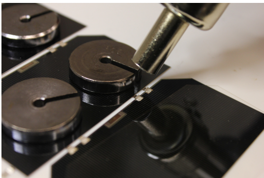
Figure 2: MXL's heritage method of solar cell stringing.
