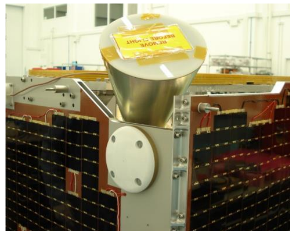
Figure 5: TDS-1 Zenith GNSS Antenna
