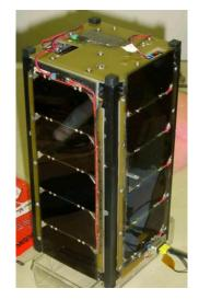
Figure 1: ION, the University of Illinois' first nanosatellite
