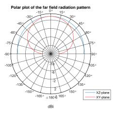
Figure 13: Polar plot of the far field radiation pattern of the PIFA at its resonance frequency.
