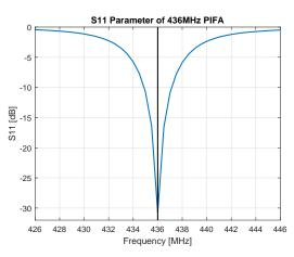
Figure 11: Reflection coefficient of the PIFA antenna.
