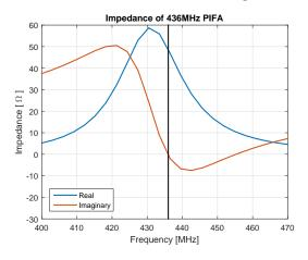
Figure 8: Impedance plot of the second antenna design.
