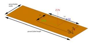
Figure 3: Structure of the PIFA.
