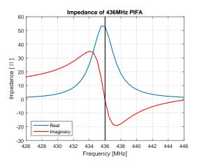
Figure 10: Real and imaginary impedance of the PIFA antenna.
