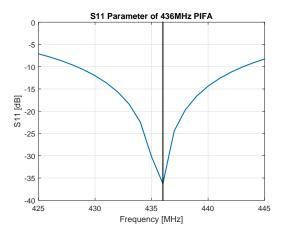
Figure 6: Return loss of the second antenna design.
