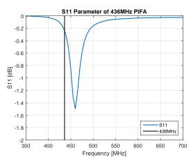
Figure 5: Reflection coefficient of the first antenna design.
