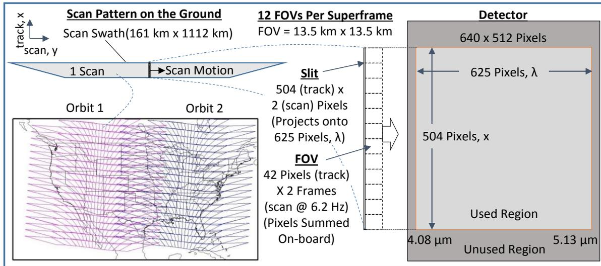
**Figure 4. CIRAS uses pixel and frame binning and an adjustable scan rate to achieve 3km (Zoom) or 13.5 km (Global) FOVs from any orbit (13.5 km FOV from 600km orbit altitude shown).**
