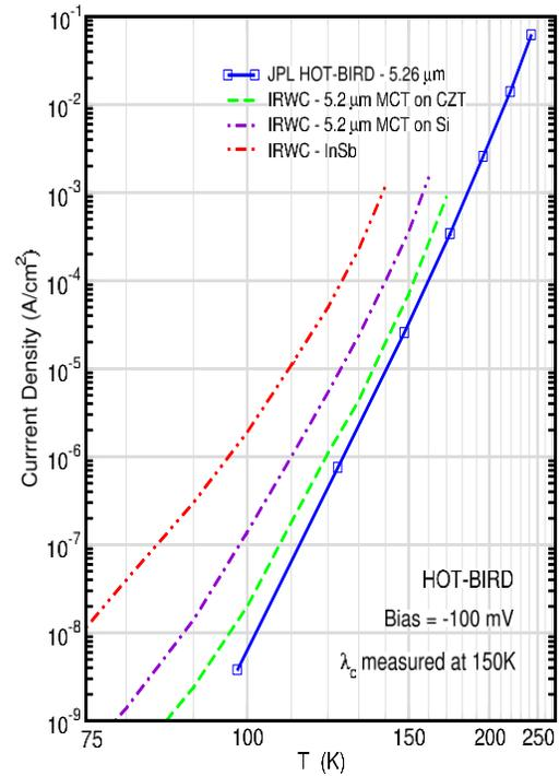
**Figure 7. Dark current vs temperature for a JPL HOT-BIRD device compared to InSb and MCT.**
