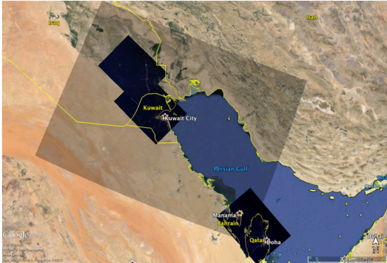
Figure 3. The Persian Gulf Region with Overlaid AeroCube Camera Fields of View. 3 Frames from the 11 May 2015 AC-5 NFOV Camera Flyby Experiment are Depicted with the Larger 11 July 2014 AC-4 MFOV Camera Footprint Superimposed.
