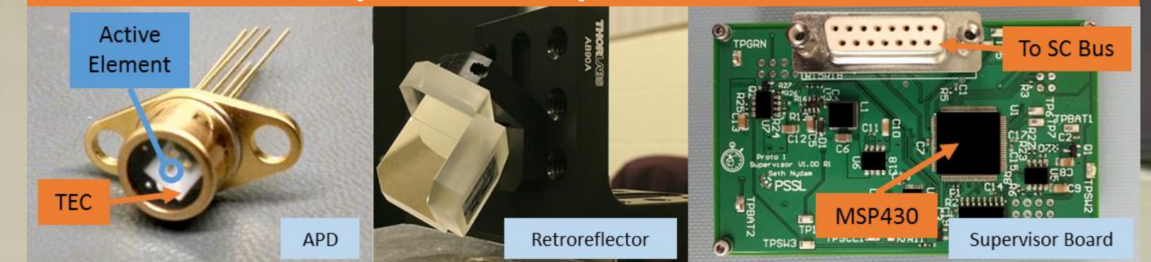
Fig. 8 APD with thermal electric cooler (TEC), Retroreflector, and the engineering version supervisor assembly with power and data interface to the spacecraft (SC) bus.
