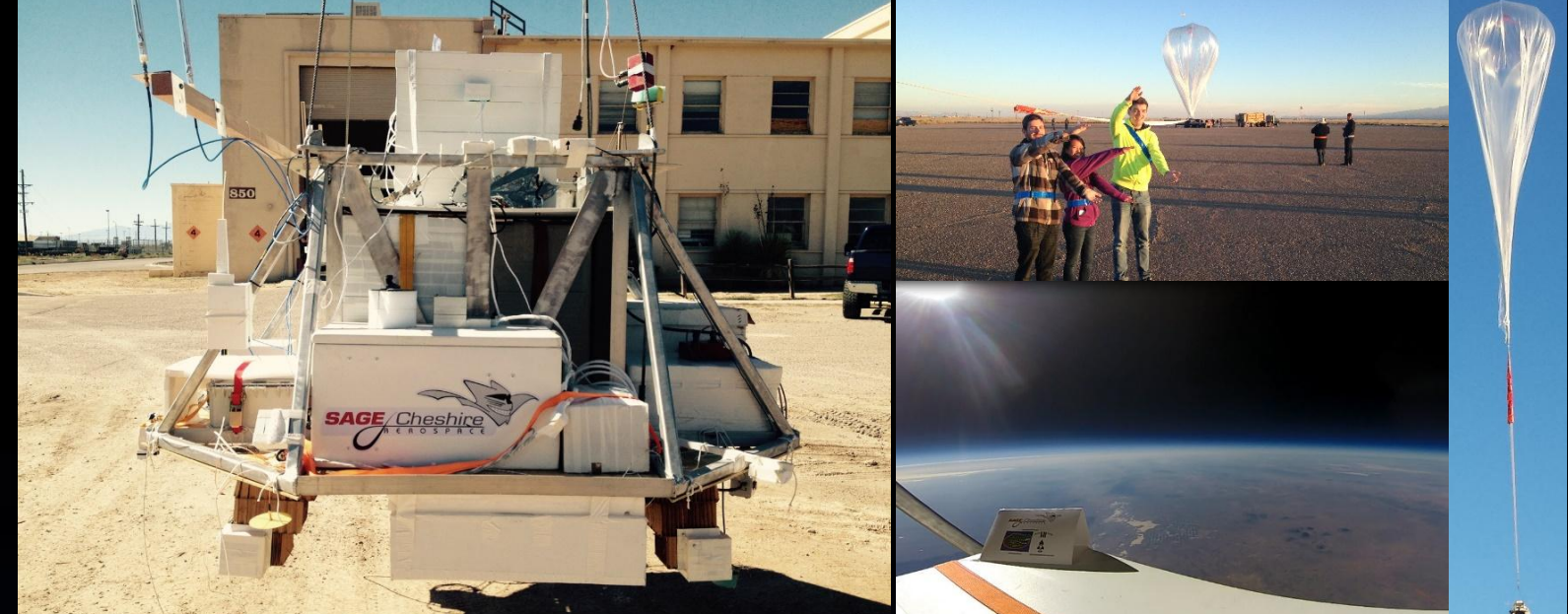
Fig. 9 Sage Cheshire high altitude balloon launch. Successful operation of OPTI in near space environment (no laser or time transfer test was performed, CSAC clock cycles counted).
