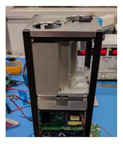
Figure 3 : Payload qualification model. From bottom to top: electronic, piezo-stage and telescope.
