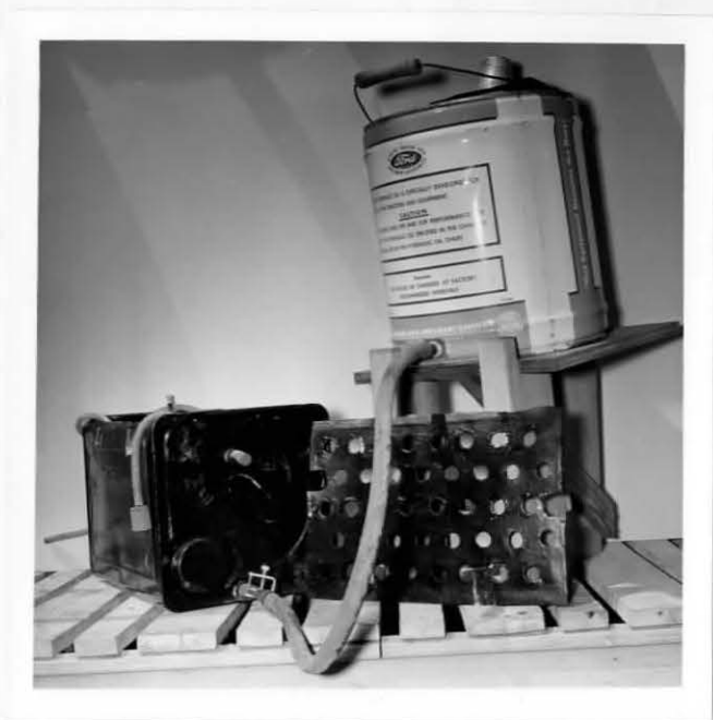
Figure 1. Five-gallon culture solution tank made from honey can showing the inlet and overflow tubes on the handle end, stone bubbler, lid with holes for split corks, and funnel bucket on stand attached to inlet tube for purposes of filling tank.
