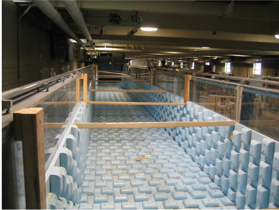
Figure 3-4. Block boundary roughness material
