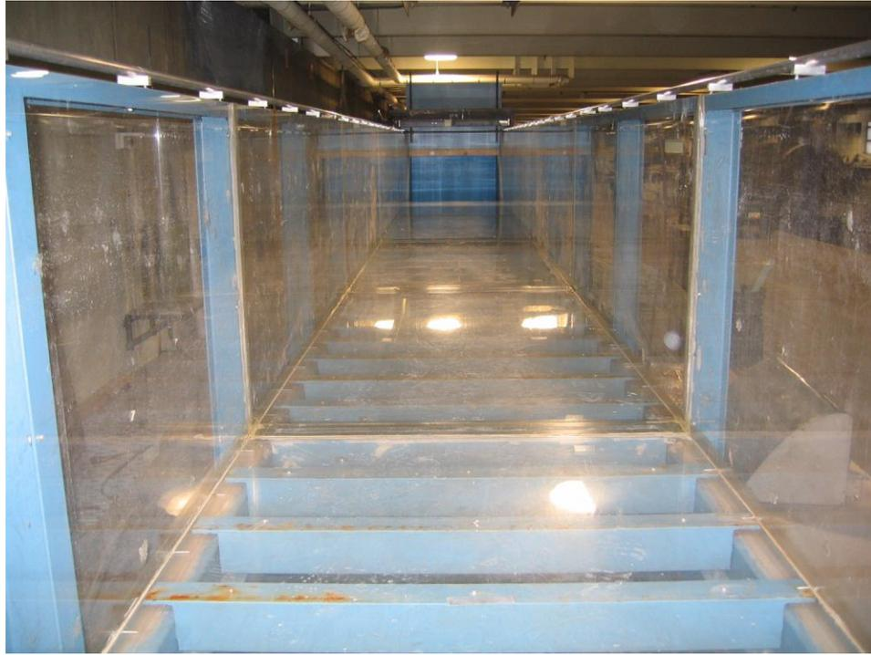
Figure 3-2. Acrylic boundary roughness material
