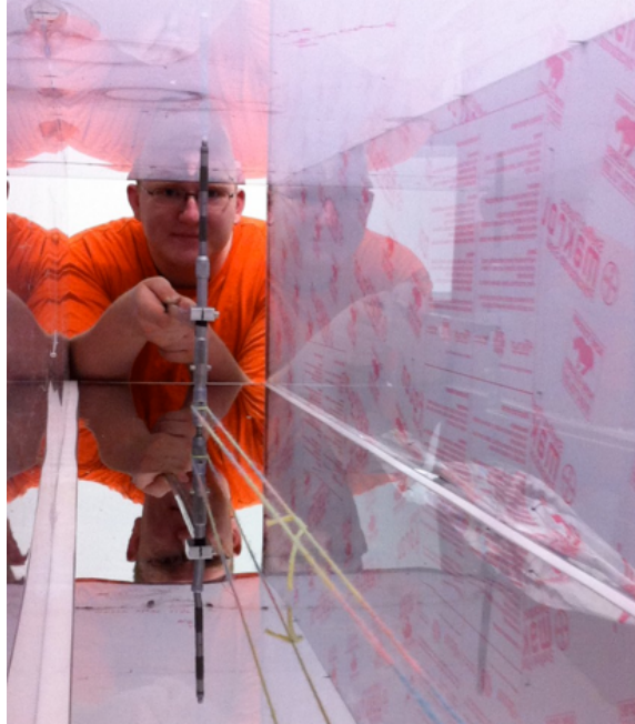
Fig. 4.2: Photograph of as-built geometry measurement procedure.
