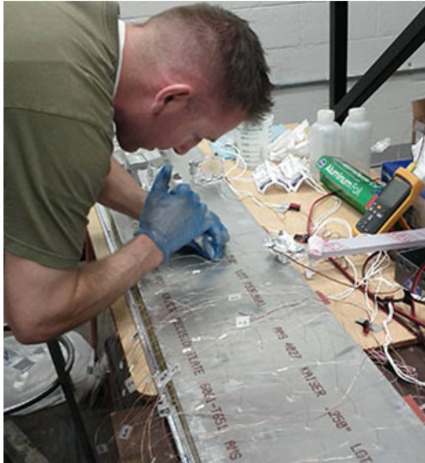
Fig. 3.8: The installation of the plate thermocouples using a syringe to place the epoxy to hold the thermocouples in place.
