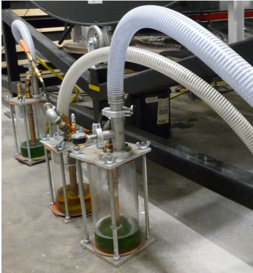
Fig. 3.10: A photograph of a seeding canister, similar to a Laskin nozzle.
