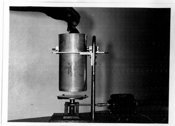
Figure 1. The mite brushing machine used for removing mites from leaves
