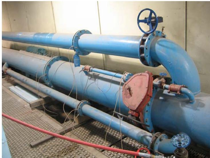
Fig. 2-7. Supply piping for the culvert (0.3 m pipe)
