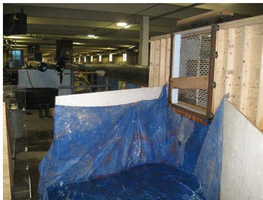
Fig. 2-6. Tail water box outlet
