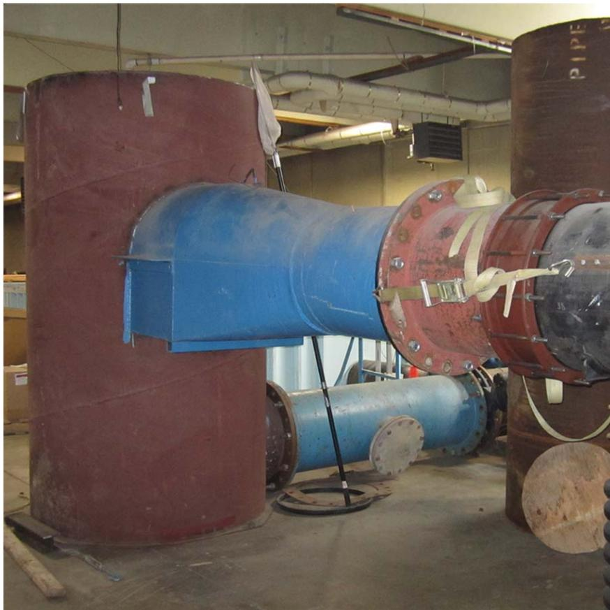
Fig. 2-4. Head tank and the flexible coupler
