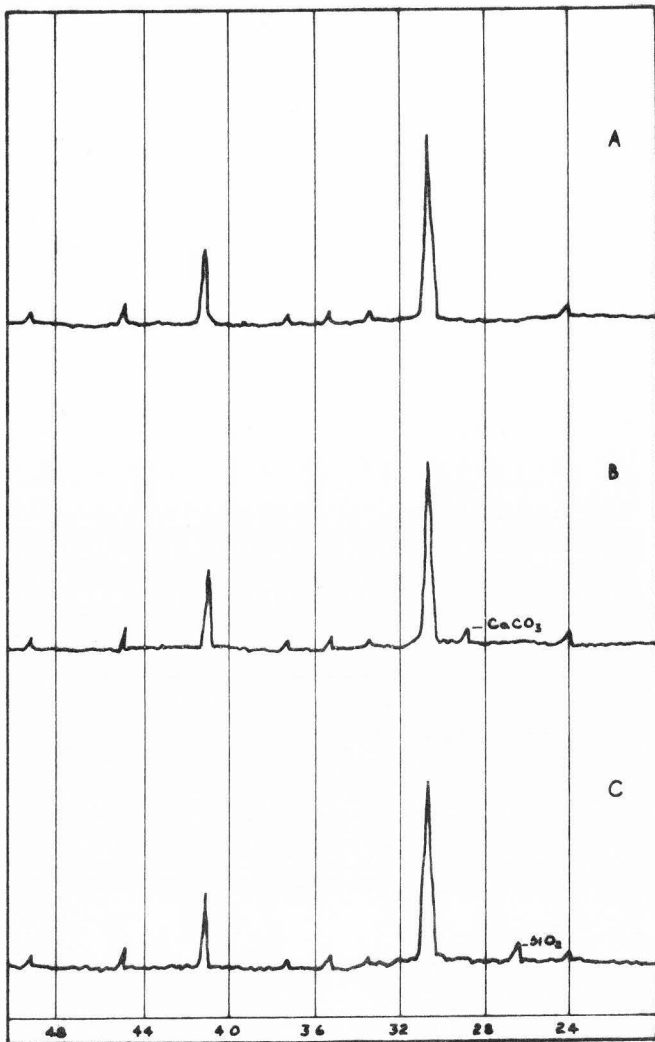
Figure 8. X-ray diffractograms from Logan Canyon Section. (A) Sample number 36, pure dolomite, (B) Sample number 106, dolomite with a minor amount of calcite, and (C) Sample number 60, dolomite with a minor amount of quartz.
