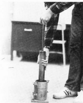
Figure III-5. Proctor cylinder ( 1/30 \text{ ft}^3 volume ( 9.40 \times 10^{-4} \text{ m}^3 )) and 5.5 lb (24.47 N) hammer.
