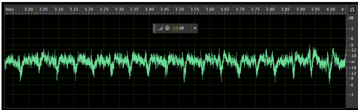
Fig. A13. Model #2d nappe vibration audio recording with one splitter, 0.34 \text{ ft}^2/\text{s} (x-axis = time in seconds, y-axis = decibel measurement)
