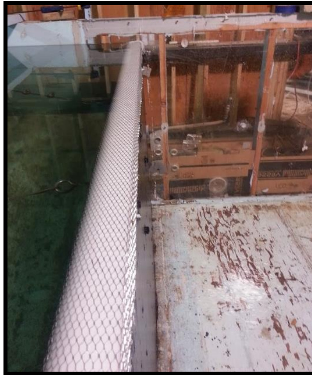
Fig. 14. Model #1b expanded metal roughness
