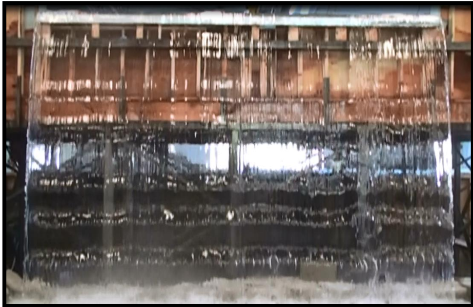
Fig. 1. Visible waves due to nappe oscillation
