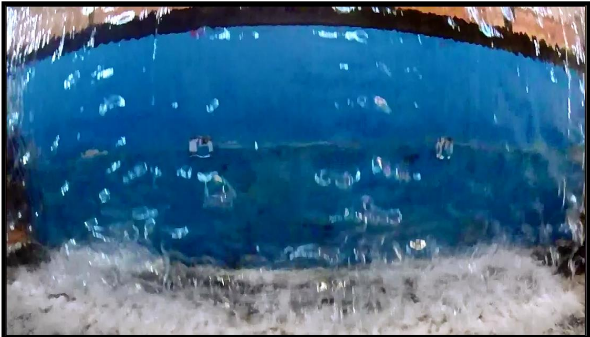
Fig. 67. Model #3b out of phase nappe waves
