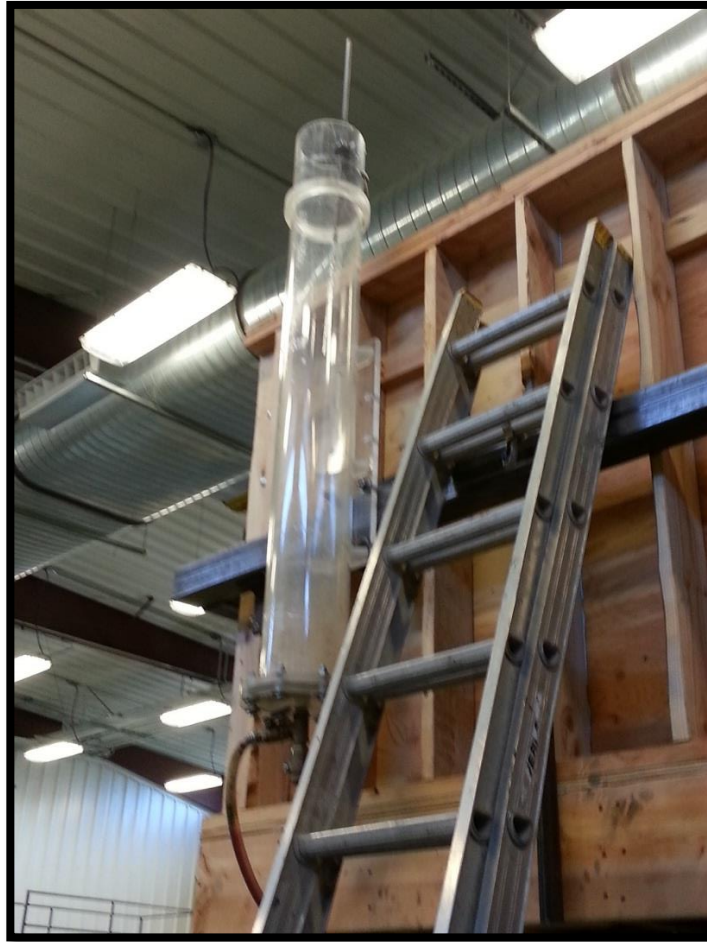
Fig. 13 Model #3 reservoir head point gauge
