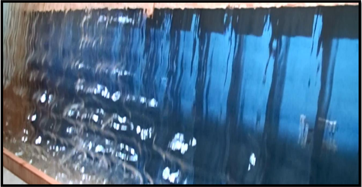
Fig. 71. Model #3d nappe vibration, 0.36 \text{ ft}^2/\text{s}
