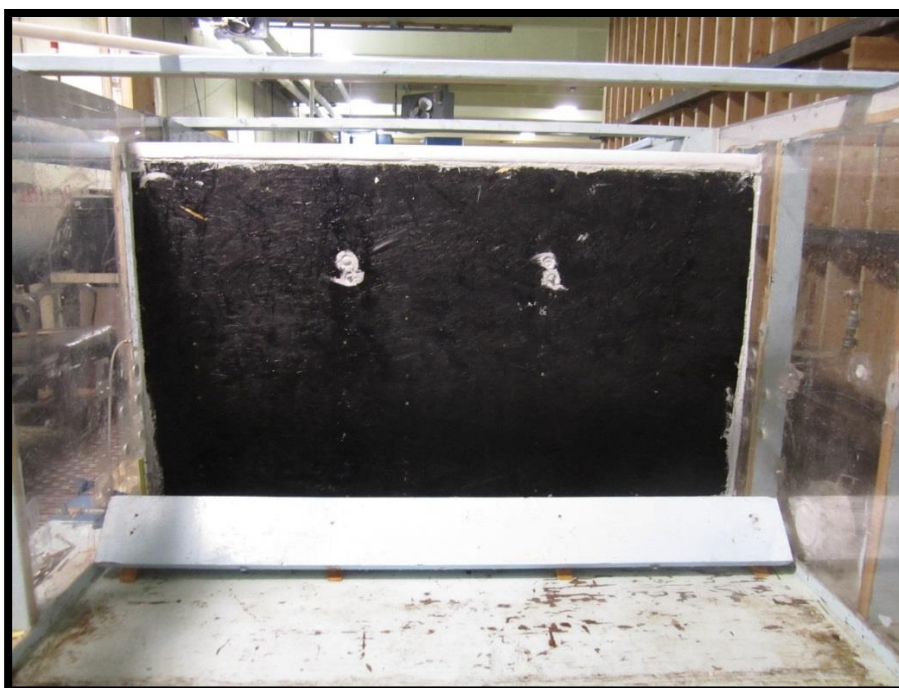
Fig. 17. Model #1f wooden impact plate on the apron
