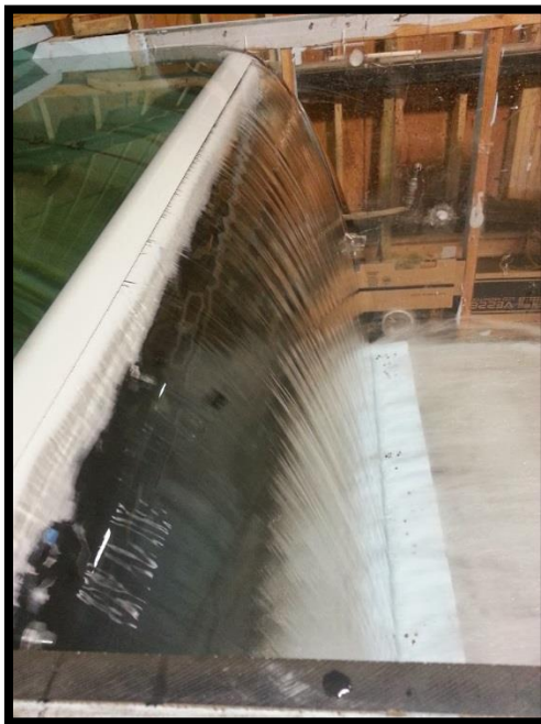
Fig. 44. Model #1g nappe deflection angle
