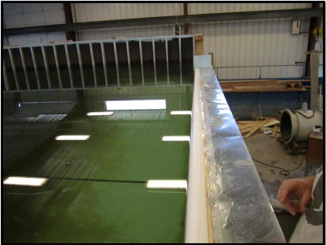
Fig. 18. Model #2b weir with rounded section upstream
