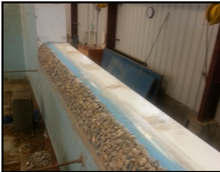
Fig. 21. Model #3b and #3d stone roughness
