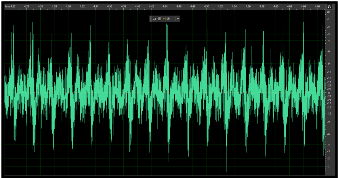
Fig. B5 Model #3a nappe vibration audio recording (grate impact), 0.25 \text{ ft}^2/\text{s} (x-axis = time in seconds, y-axis = decibel measurement)
