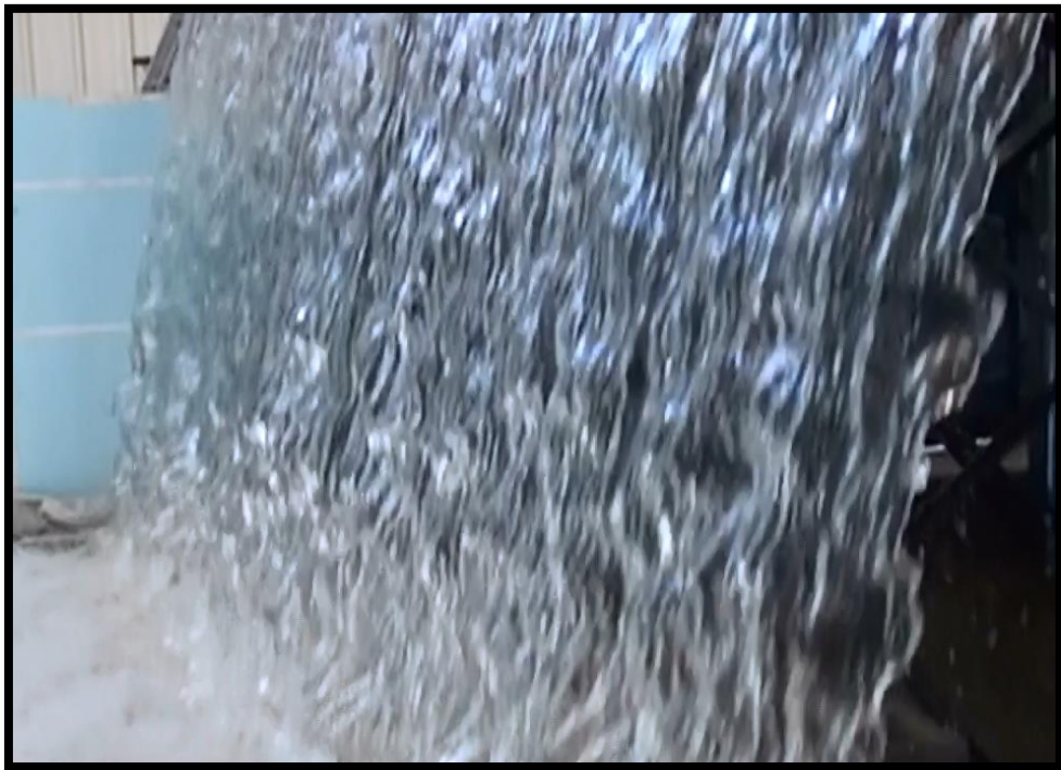
Fig. 54. Model #2c nappe appearance
