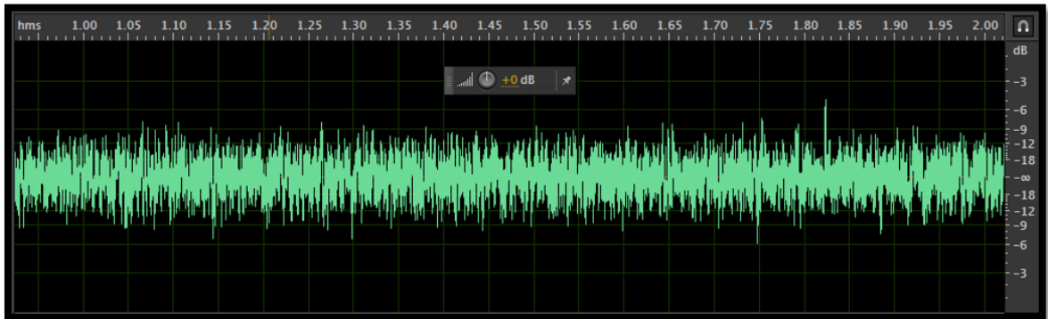
Fig. A25. Model #2d nappe vibration audio recording with three splitters, 0.47 \text{ ft}^2/\text{s} (x-axis = time in seconds, y-axis = decibel measurement)
