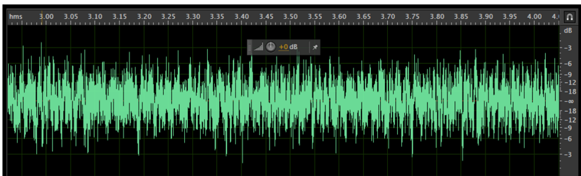
Fig. A24. Model #2d nappe vibration audio recording with two splitters, 0.47 \text{ ft}^2/\text{s} (x-axis = time in seconds, y-axis = decibel measurement)
