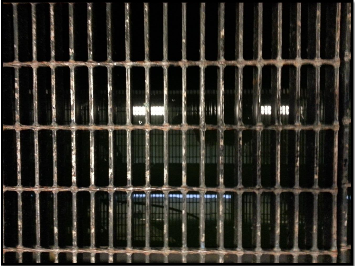
Fig. 10. Model #3 nappe impact grate
