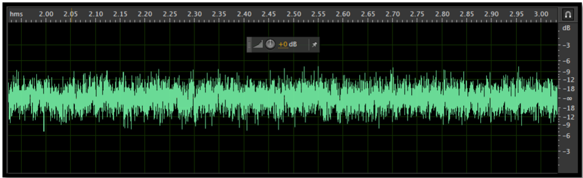
Fig. A12. Model #2c nappe vibration audio recording, 0.34 ft 2 /s (x-axis = time in seconds, y-axis = decibel measurement)
