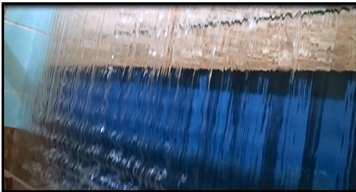
Fig. 76. Model #3h nappe appearance, 0.36 \text{ ft}^2/\text{s}
