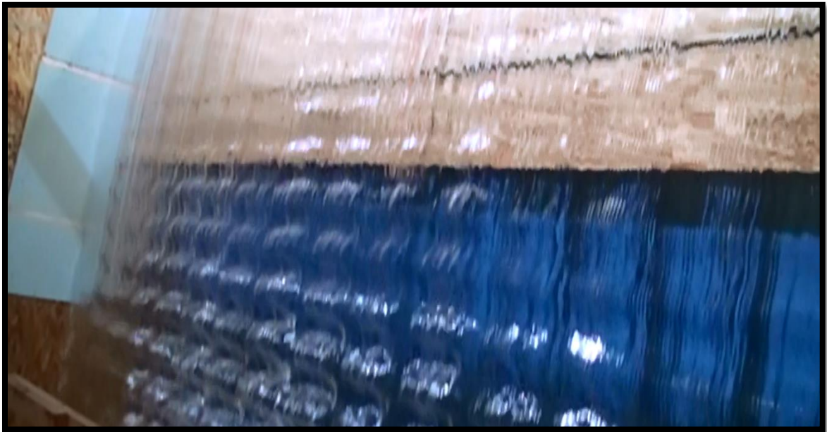
Fig. 75. Model #3g-b nappe appearance, 0.36 ft 2 /s
