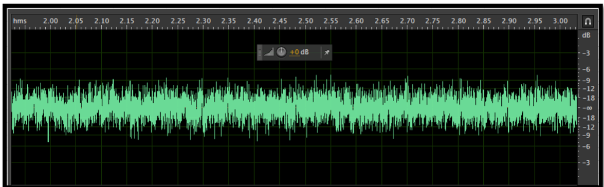
Fig. 52. Model #2c nappe vibration audio recording, 0.34 \text{ ft}^2/\text{s} (x-axis = time in seconds, y-axis = decibel measurement)
