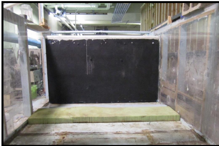
Fig. 16. Model #1d open-cell foam pad on the apron (flume floor)
