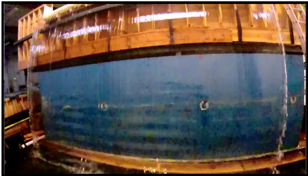
Fig. 60. Model #3a impacting on the metal grating, 0.31 \text{ ft}^2/\text{s}
