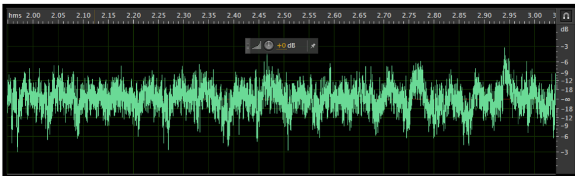
Fig. A14. Model #2d nappe vibration audio recording with two splitters, 0.34 \text{ ft}^2/\text{s} (x-axis = time in seconds, y-axis = decibel measurement)
