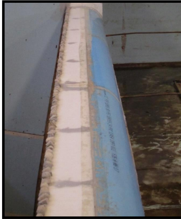
Fig. 25. Model #3f stone roughness
