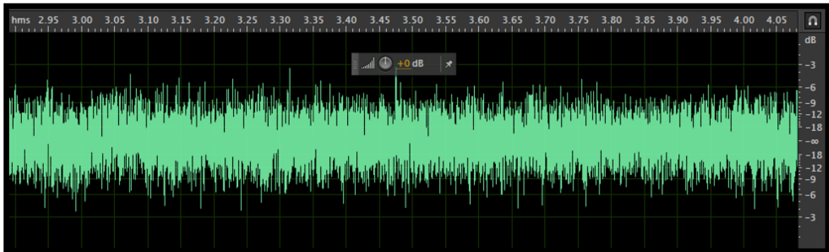
Fig. A7. Model #2c nappe vibration audio recording, 0.28 \text{ ft}^2/\text{s} (x-axis = time in seconds, y-axis = decibel measurement)
