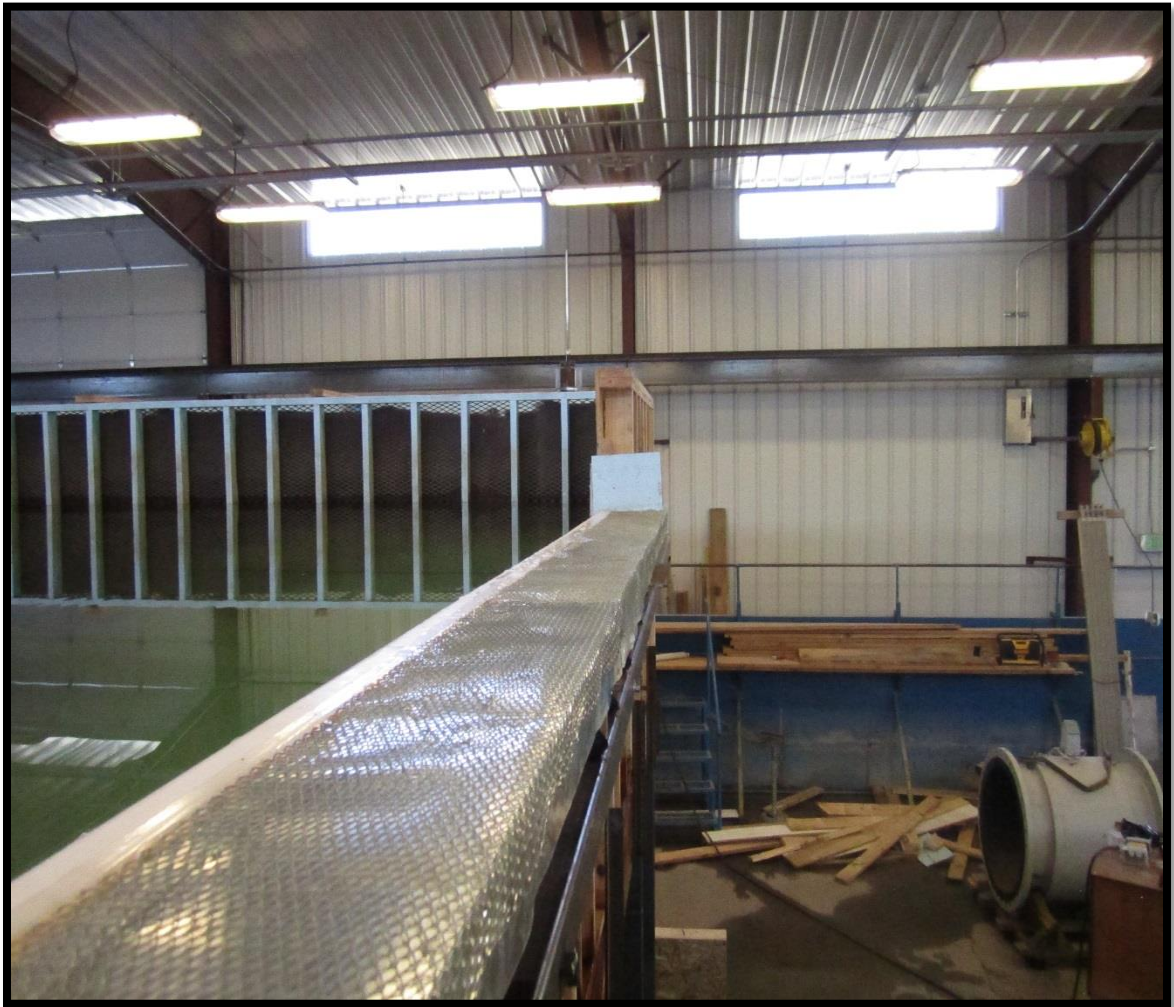
Fig. 19. Model #2c expanded metal roughness
