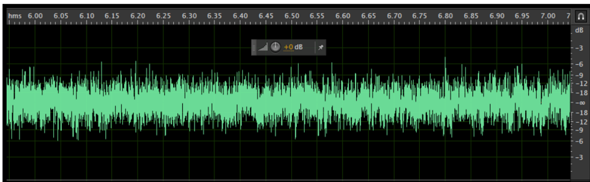
Fig. A5. Model #2d nappe vibration audio recording with three splitters, 0.22 \text{ ft}^2/\text{s} (x-axis = time in seconds, y-axis = decibel measurement)
