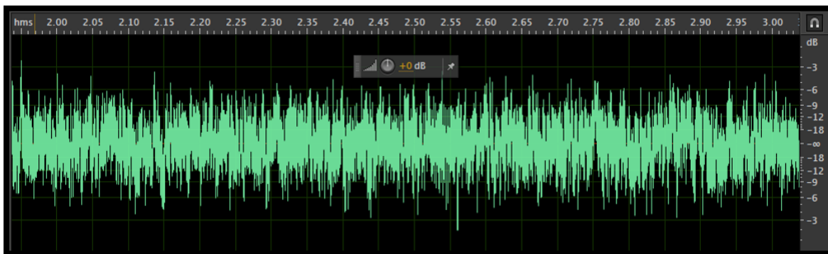
Fig. A17. Model #2c nappe vibration audio recording, 0.40 \text{ ft}^2/\text{s} (x-axis = time in seconds, y-axis = decibel measurement)
