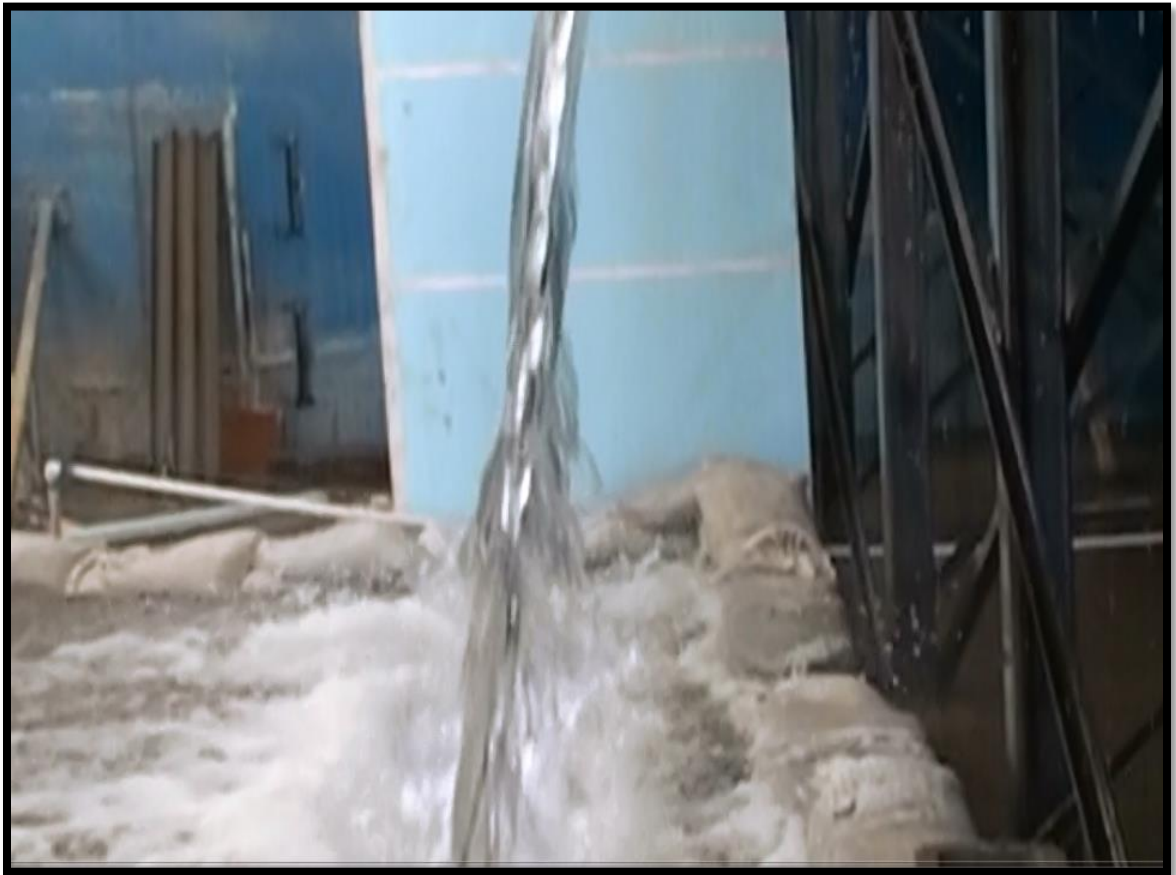
Fig. 48. Model #2b sheet breakup at the bottom of the nappe
