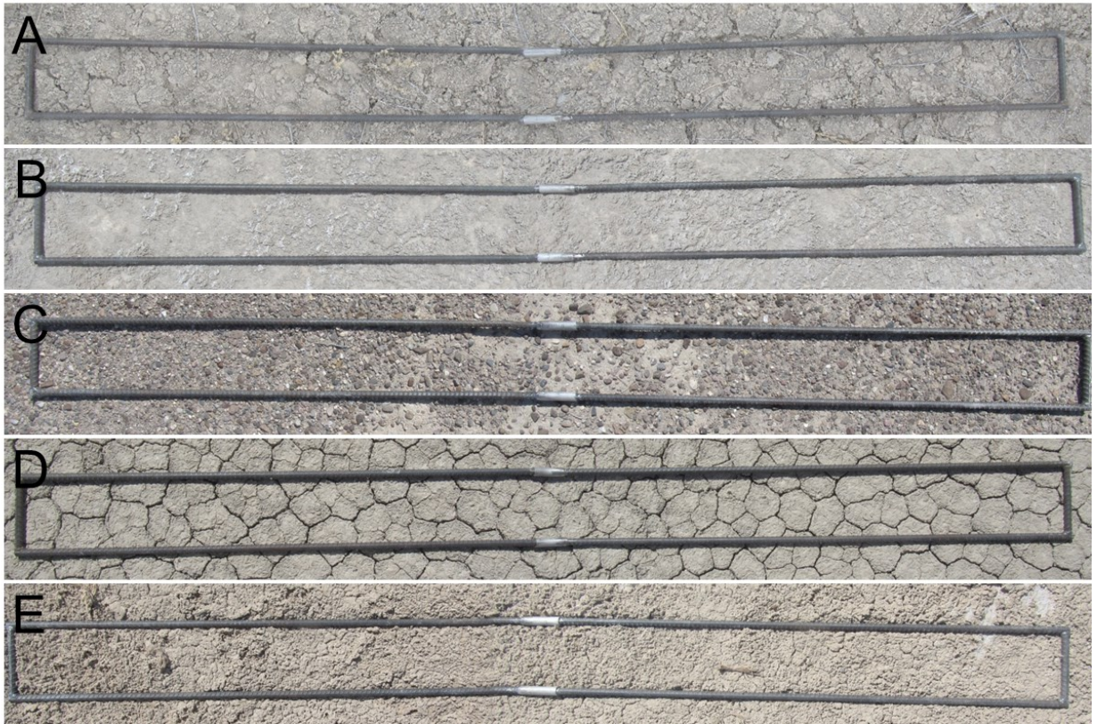
Fig. 4-4. Photos of representative sites from each soil surface type. From top to bottom: biological crust (A), hard salt crust (B), surficial rock fragments (C), hard physical crust (D), and weak physical crust (E). The steel frame in each photo is equal to the wind tunnel footprint.
