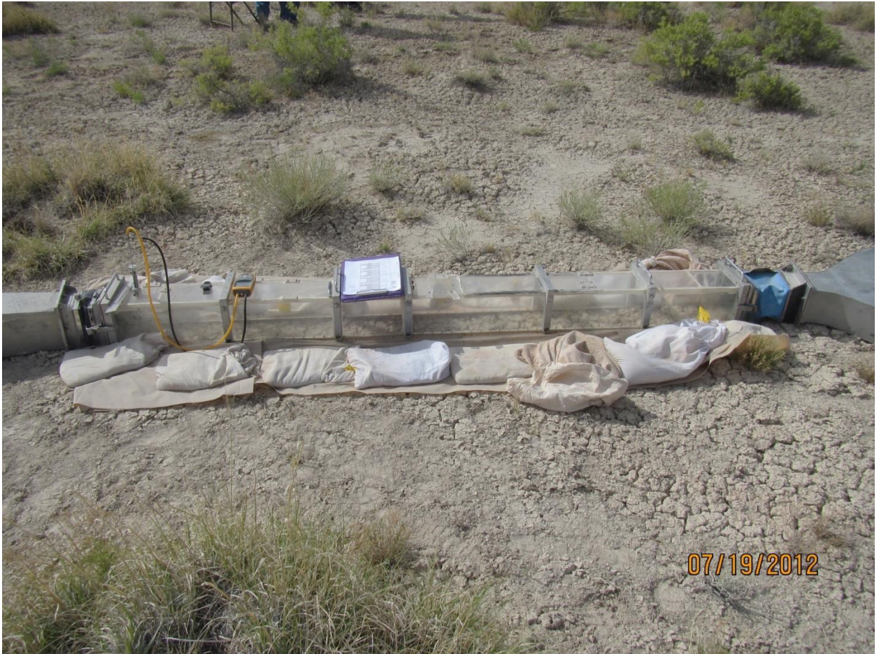
Fig. 4-2. Clear plastic main working section of the portable wind tunnel used to measure TFV. Honeycomb flow straightener is located to the right. The expansion chamber and filter (not in photo) are located to the left. Wind travels along wind tunnel from right to left. Yellow and black tubes connect the pitot tube inside the wind tunnel to the Fluke 922 airflow meter/micromanometer.
