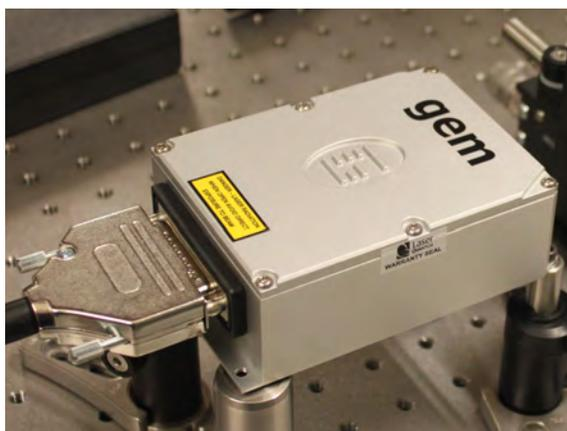
Fig. 5.1: Image of the 575mW ND:YAG, frequency doubled (532 nm) laser used in the PTR system.
