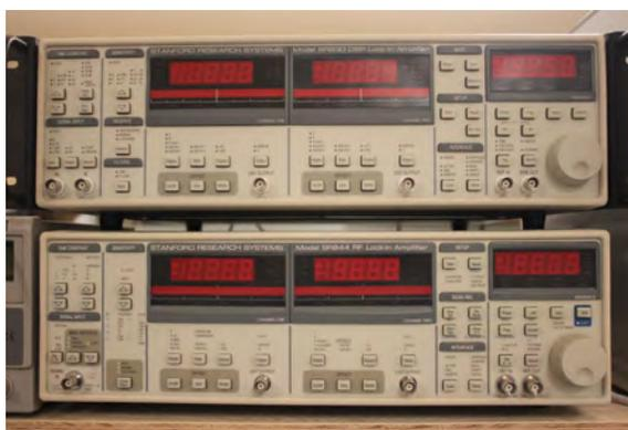
Fig. 5.5: Image of the lock-in amplifiers used in the PTR system to filter out noise and amplify the detector signal at the modulation frequency.
