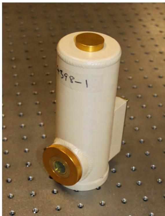
Fig. 5.3: Image of the Kolmar Technologies Mercury Cadmium Telluride infrared radiation detector used in PTR system.
