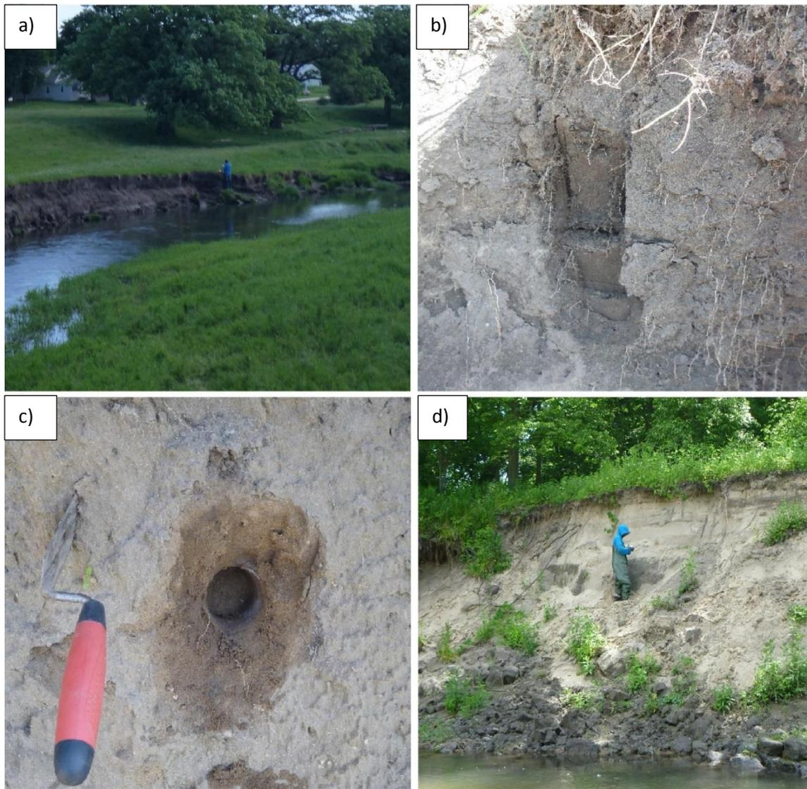
Figure 3.2. Grain size and bulk density campaign, summer 2013. a) banks upstream the North Branch, b) vertical bank from where grain size samples were collected, c) vertical bank after collecting bulk density sample, d) sandy banks at Rushford Creek.
