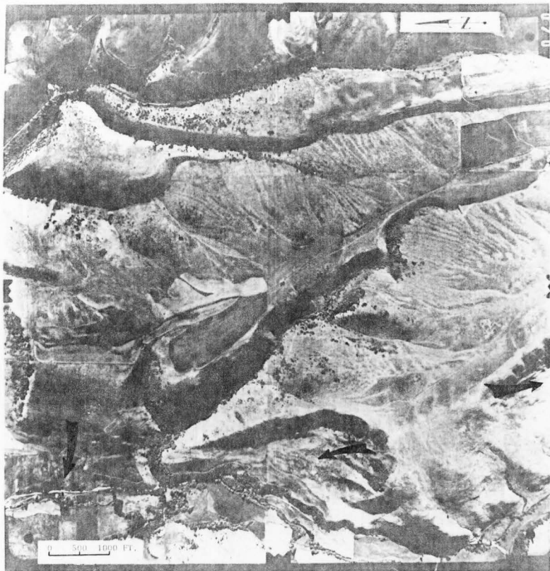
Figure 3-13. Low-sun-angle view of slides near Avon, Utah, (after Cluff, Glass, and Brogan, 1974).
