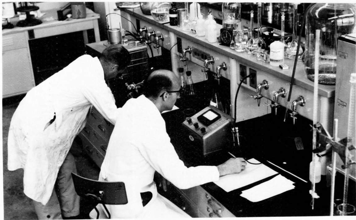
Figure 6. Abbe-type refractometer with constant temperature bath at left Beckman pH meter at right
