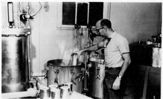
Figure 1. a. Preparing, weighing, and syreping the fruit for processing b. Sealing the cans in the Pacific No. 1 Semi-automatic closing machine c. Cooking the fruit in the Master Retort 100
