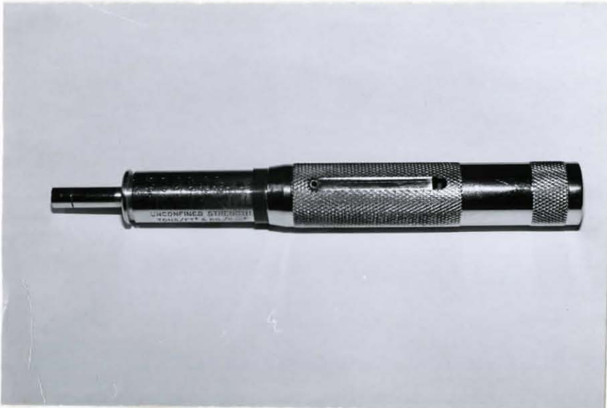
Figure 2. Pocket penetrometer that was used for measurement of soil crust resistance to penetration.
