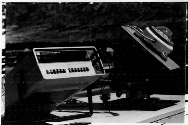
Fig. 33. Instrumentation used to measure diffuse irradiance on various tilted surfaces--digital voltmeter, tilt platform, and star pyranometer.
