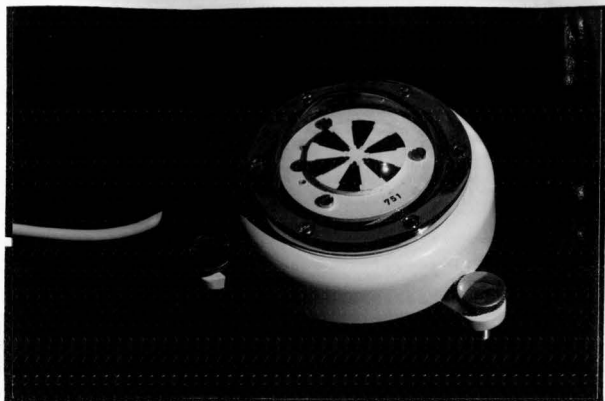
Fig. 7. Black and white star pyranometer used throughout the study.
