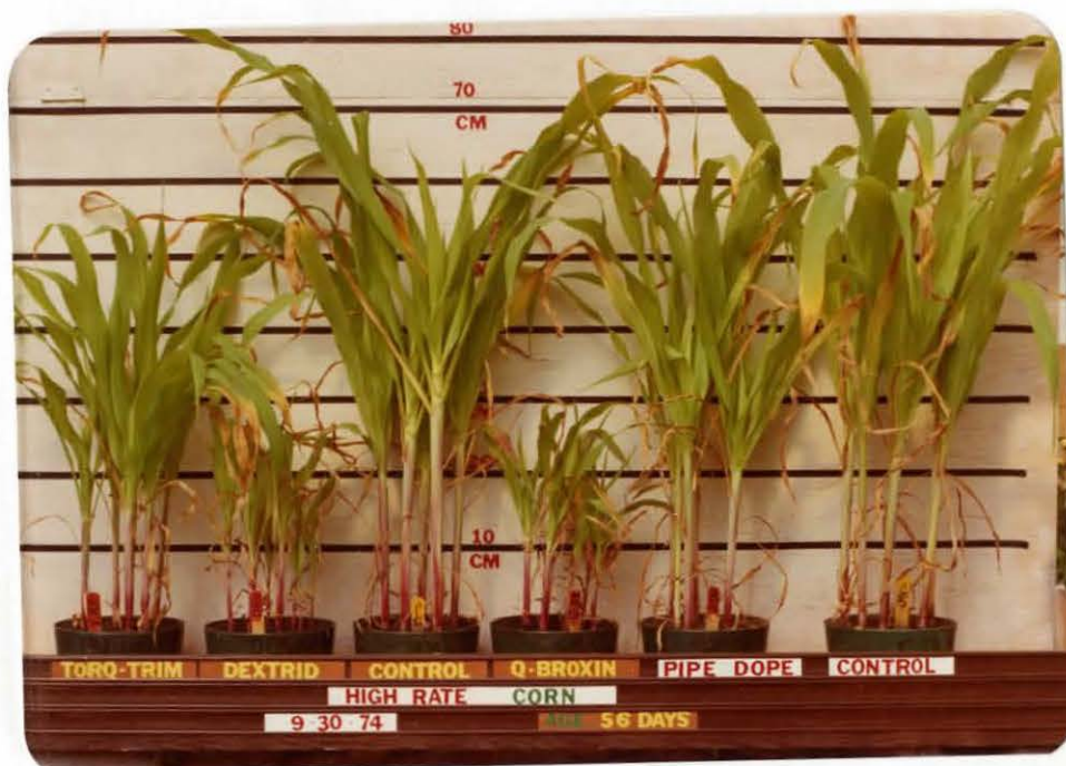
Figure 14. Example of four materials and their affect on corn growth. Phase I, Part A, Corn. Torq-Trim, Dextrid and Q-Broxin all reduced plant growth. The effect of pipe dope was small.
