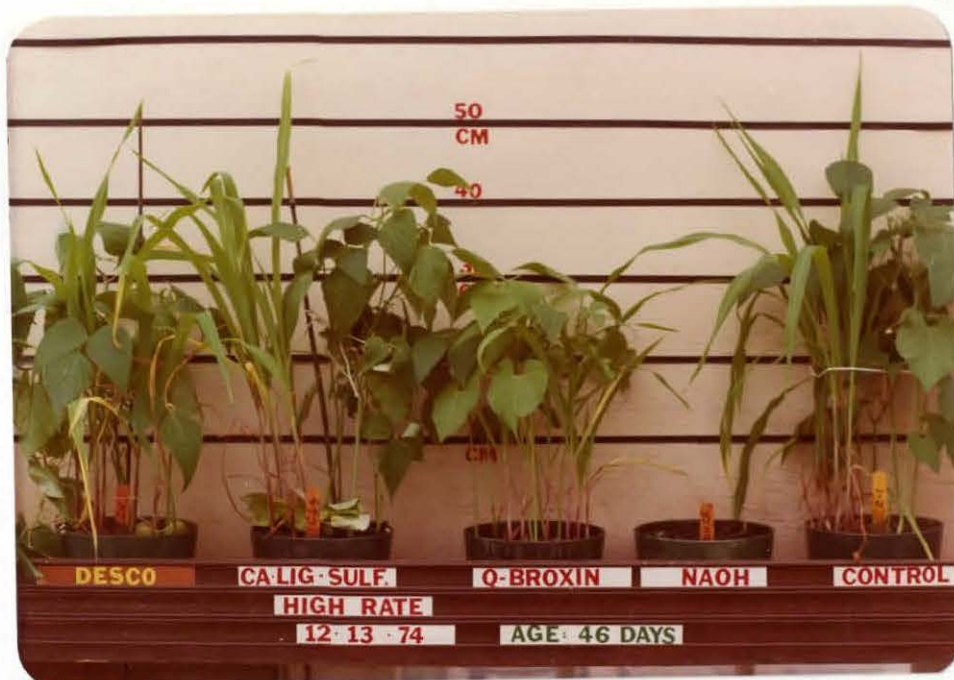
Figure 17. Second planting of some Part A soil treatments. Phase I, Part A-2. Sodium hydroxide hindered any germination. Q-Broxin still hinders growth of both beans and corn. The effect of calcium lignosulfonate and Desco were less obvious.
