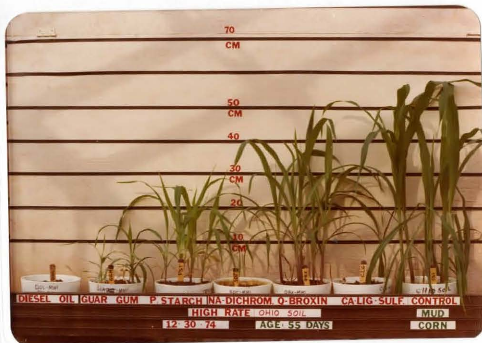
Figure 30. Plant growth in selected treatments (high rate) on the acid Miamian (Ohio) soil. Phase I, Part B. No growth of corn occurred in calcium lignosulfonate (+ sodium hydroxide), diesel oil or sodium dichromate. Growth was successively better in Guar gum, pregelatinized starch, and Q-Broxin.
