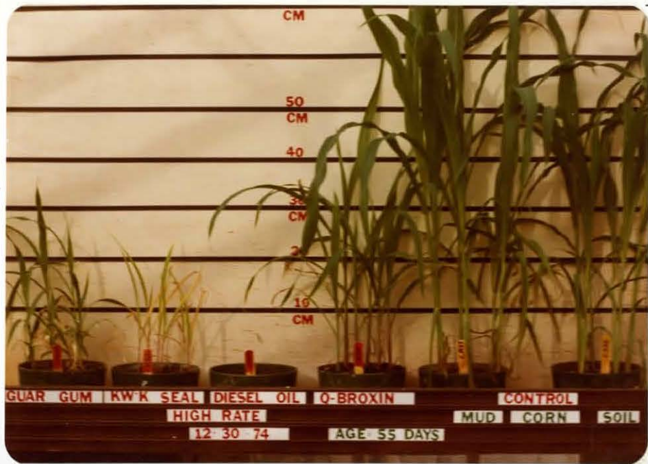
Figure 23. Selected treatments at high addition rates. Guar gum, Kwik-Seal, diesel oil, and Q-Broxin. Phase I, Part B, Corn.
