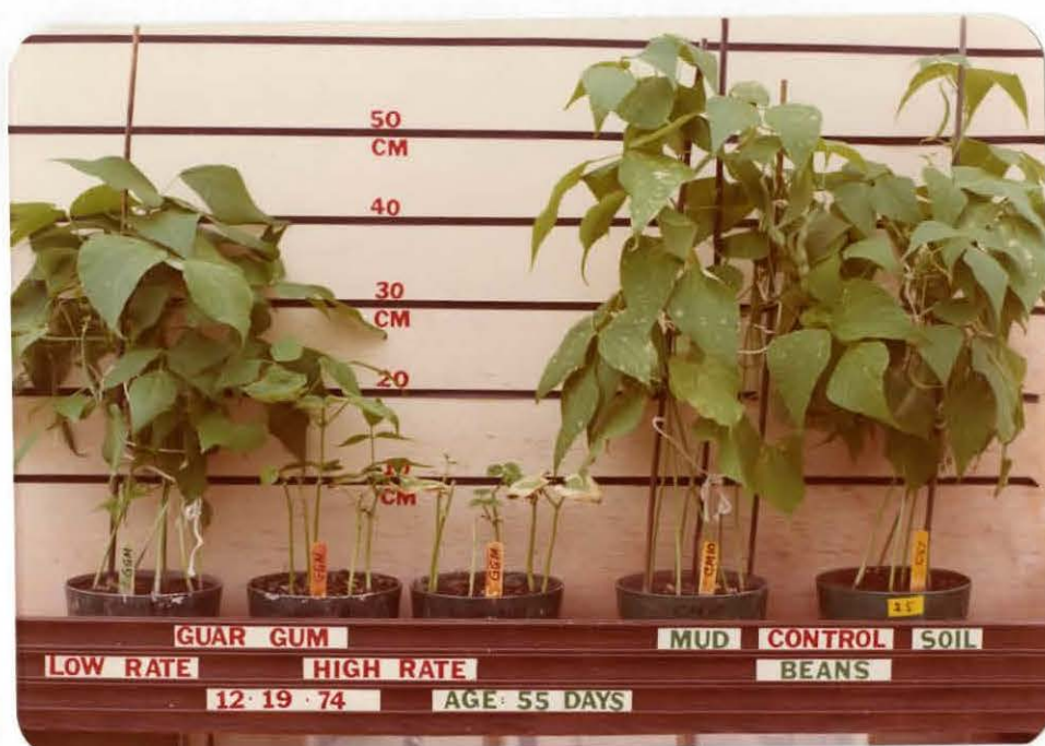
Figure 20. Guar gum at the following concentrations: high rate = 6 lb/bbl (24.5 g/1.6 l); low rate = 1 lb/bbl (4.09 g/1.6 l). Phase I, Part B, Beans. Slight growth reductions occurred in low treatment rates. Severe growth retardation occurred in high level treatment rates. Leaf-edge scorch was typical on older levels.
