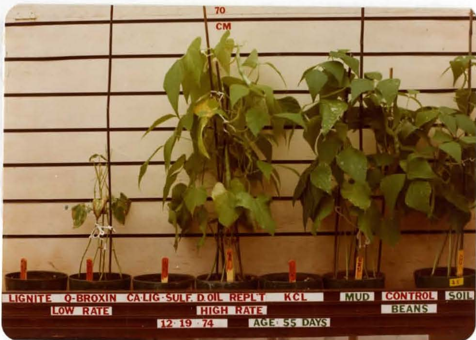
Figure 22. Selected treatments at high addition rates. Lignite (+ sodium hydroxide), Q-Broxin, calcium lignosulfonate (+ sodium hydroxide), diesel oil replacement (Drillaid 405), and Potassium chloride. Phase I, Part B, Beans.
