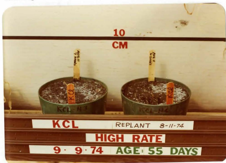
Figure 8. Potassium chloride at the high rates (30 lb/bbl or 122.78/1.8 kg of soil). Accumulation of salt occurred on top of the soil.
