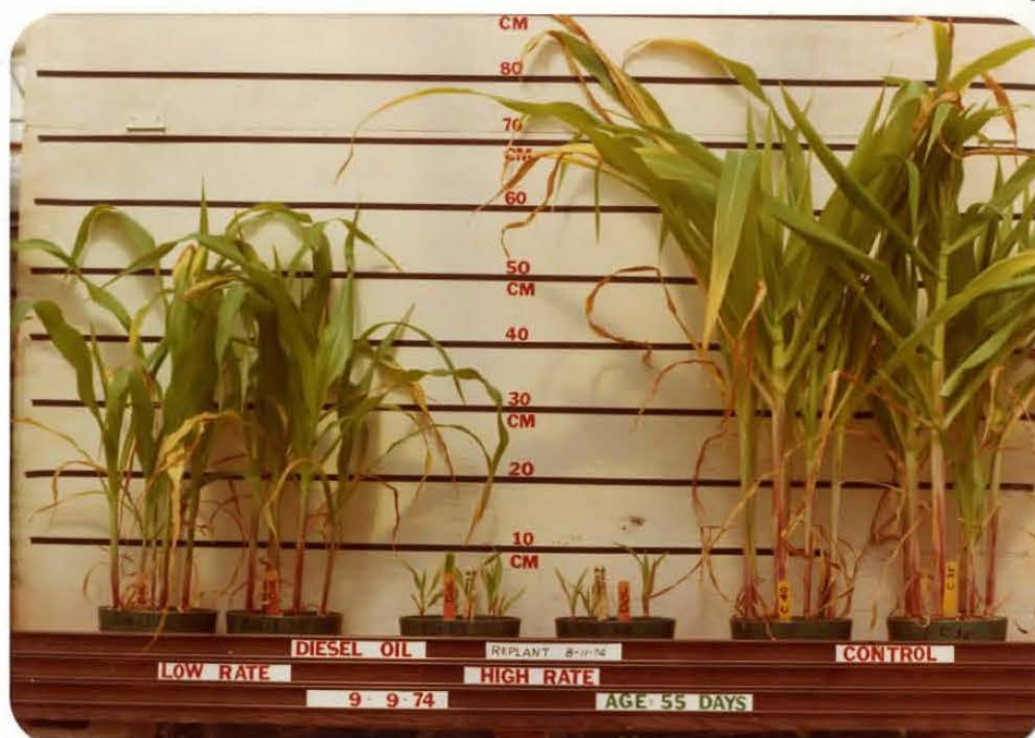
Figure 3. Diesel oil at the following concentrations: high rate = about 35 lb/bbl (10% of soil weight); low rate = 3.5 lb/bbl (1% of soil weight). Phase I, Part A, Corn. Both treatment levels reduce corn growth. No germination the first planting at high rate; poor growth on replants one month later.
