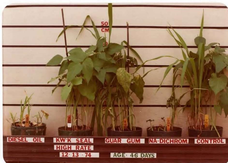
Figure 16. Second planting of some Part A soil treatments. Phase I, Part A-2. All materials shown still reduce corn growth. Kwik-Seal did not appear to reduce bean growth. The most serious growth retardation was by diesel oil and sodium dichromate treatments.
