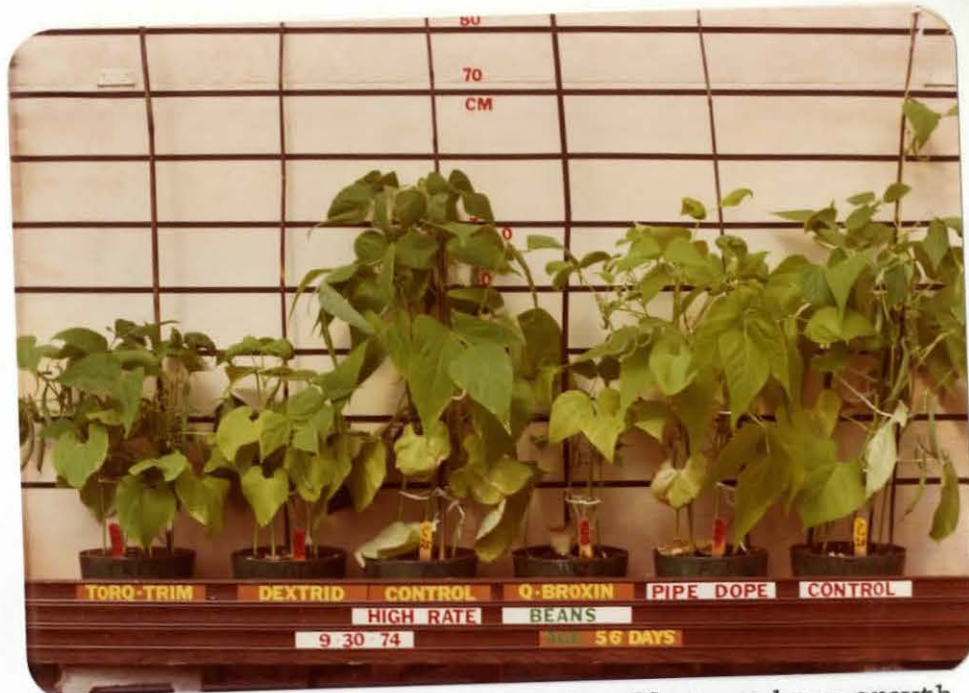
Figure 13. Example of four materials and their affect on bean growth. Phase I, Part A, Beans. Torq-Trim, Dextrid and Q-Broxin all reduced bean growth. Pipe dope had a slight effect on plant growth.
