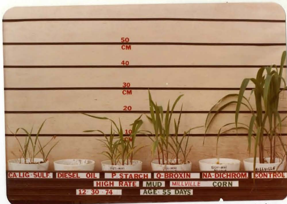
Figure 25. Corn growth in selected treatments in Millville soil (a strongly calcareous silt loam). Rates of addition per pot are the same as given in Part B for the Dagor soil. Phase I, Part B. No growth occurred in calcium lignosulfonate, pregelatinized starch, and Q-Broxin (after 55 days).
