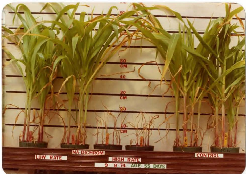
Figure 12. Sodium dichromate at the following concentrations: high rate = 3 lb/bbl (12.3 g/1.8 kg of soil); low rate = 0.5 lb/bbl (2.05 g/1.8 kg of soil). Phase I, Part A, Corn. High treatment rates almost hindered plant growth. Plants had reddish coloration and were almost dried at the age of 55 days old.
