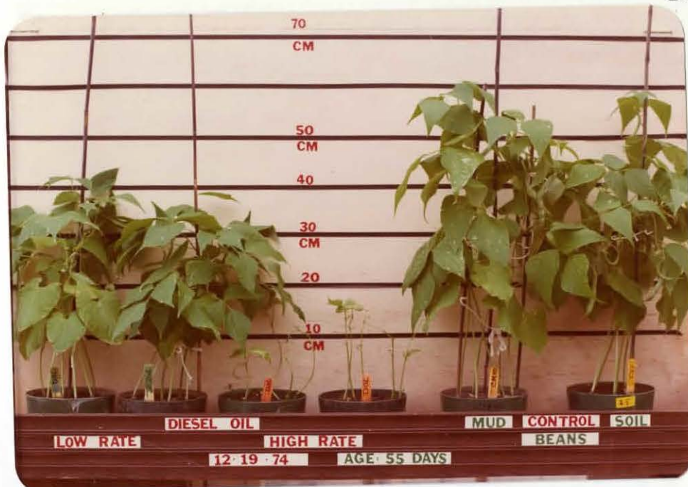
Figure 19. Diesel oil at the following concentrations: high rates = 10% by soil weight (180 g); low rate = 1% by soil weight (18.0 g). Phase I, Part B, Beans. Growth in the low treatment level was fair, but at the high rate growth was very poor. The soil-mud mixture stayed greasy in appearance.
