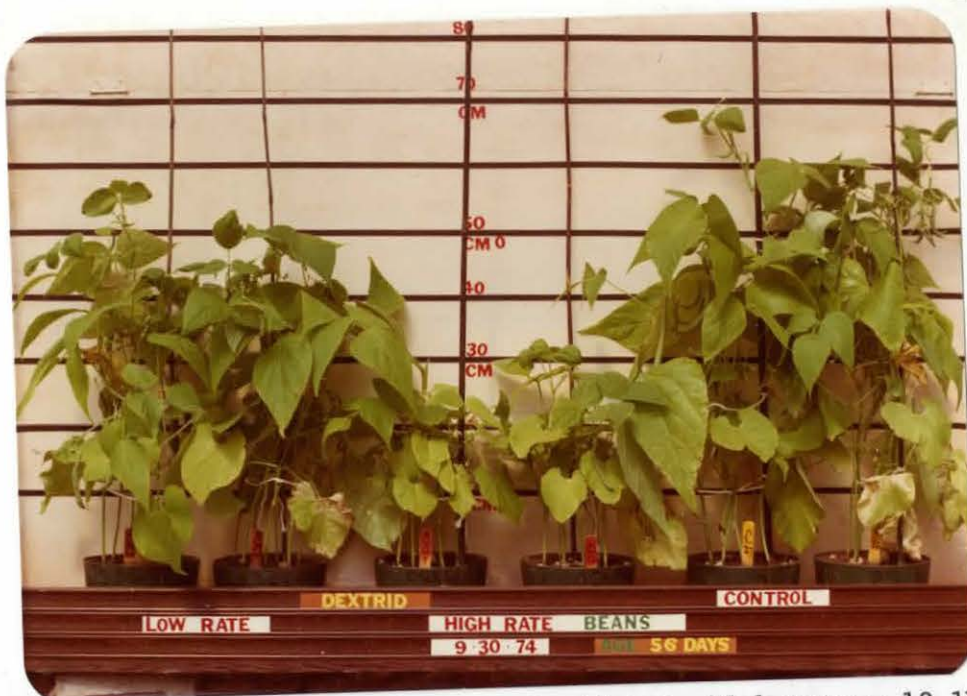
Figure 1. Dextrid at the following concentrations: high rate = 10 lb/bbl (40.9 g/1.8 kg of soil); low rate = 1 lb/bbl (4.09 g/1.8 kg of soil). Phase 1, Part A, Beans. High treatment levels reduced bean growth.
