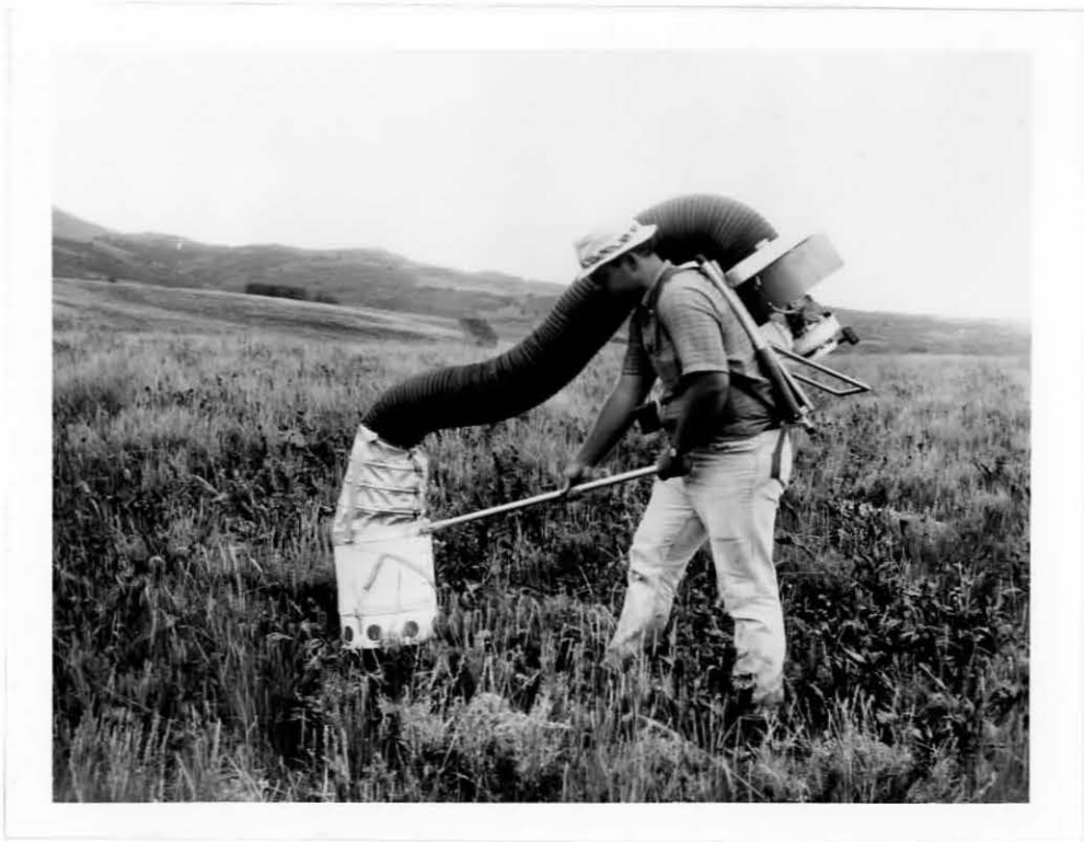
Figure 9. The author using a backpack insect sampler to make small insect collections. (Photo by Dr. J. B. Low)
