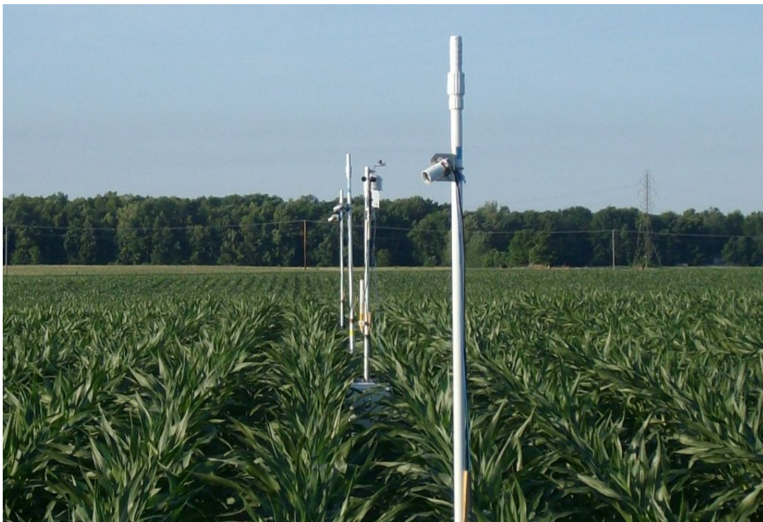
Fig. 2-2: Typical sensor arrangement in a stressed corn field. Three infrared thermometers mounted at 68 degrees (zenith angle), 22 degrees below horizontal. These sensors measured canopy temperature. The leaves in this field are beginning to roll, indicating water stress.
