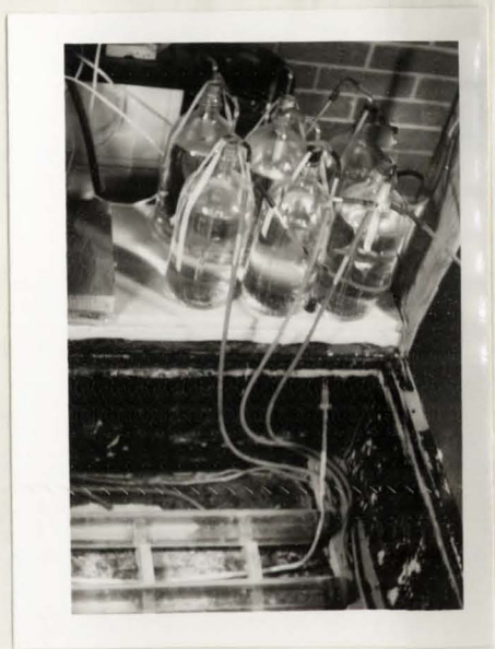
Figure 1. Bottles containing the humidifying solutions through which the air passes before reaching the plastic tubes inside the bath
