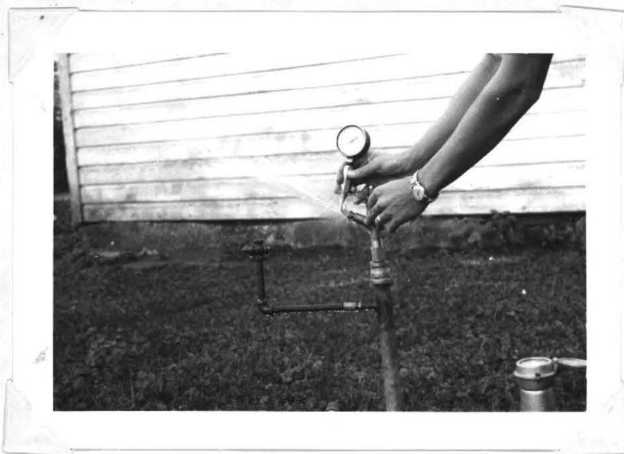
Figure 1. Method of measuring nozzle pressure with a pressure gage, and pitot tube attachment
