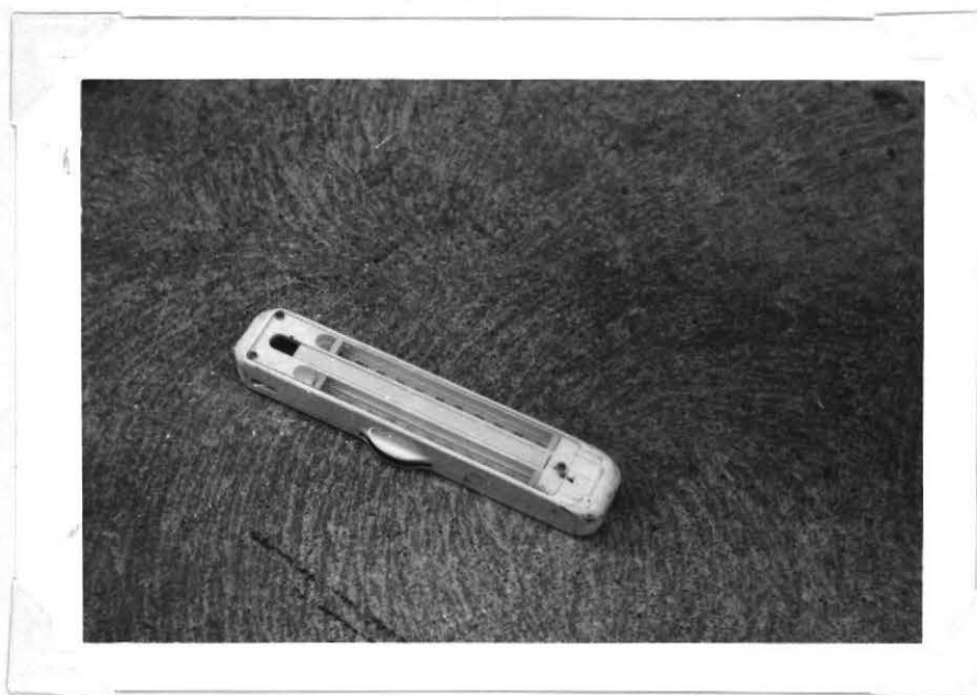
Figure 6. Hand ventilated psychrometer used to measure relative humidity
