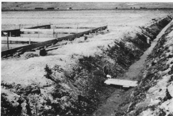
Figure 5. Plots in operation showing supporting framework, moisture tubes and ponded water. (Plots are numbered A, B, and C from left to right.)
