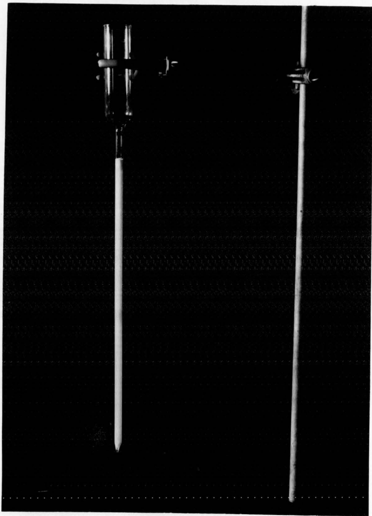
Figure 4. Resin column used for separating micronutrient elements.
