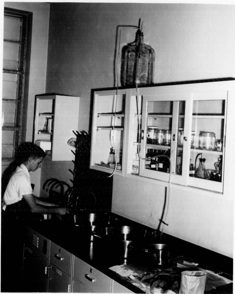
Figure 3. Leaf washing procedure showing the EDTA plus detergent wash, a tap water rinse, two distilled water rinses and one deionized water rinse.
