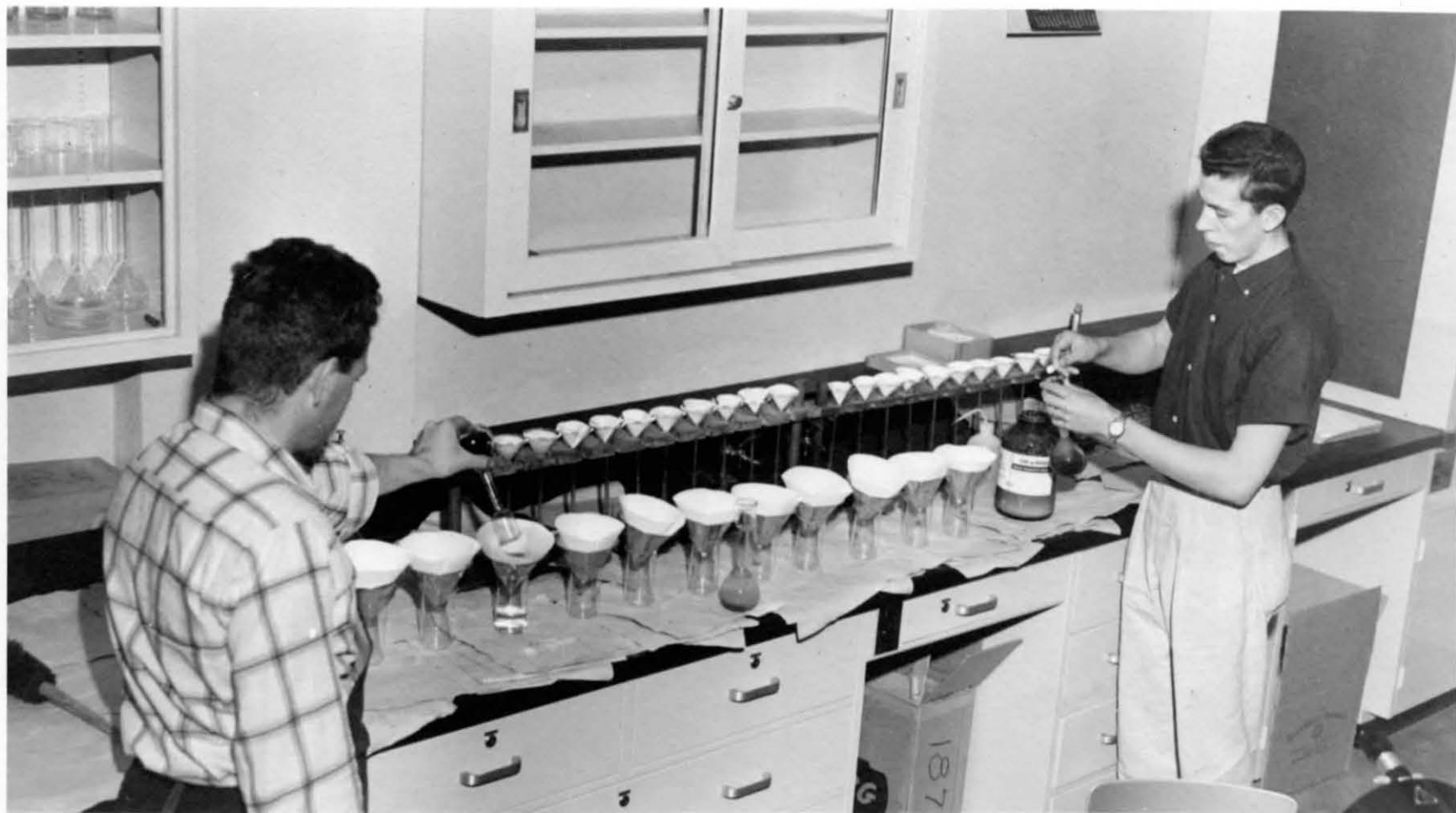
Figure 5. Clarification and filtering. Filtration for total dry solids determinations in background. Clarification and filtration for sucrose determinations in foreground.
