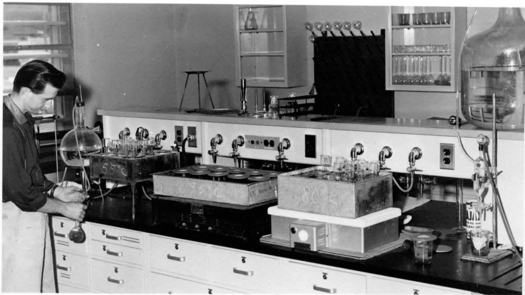
Figure 4. Digestion procedures. From left to right: 55° C. Pellet method; 55° C. Sachs-LeDocte method; 80° C. Pellet method; Sachs-LeDocte cold (20° C.) method. Swirling and rinsing for Pellet method shown on far left; 177 ml. automatic pipette for Sachs-LeDocte method shown on far right.
