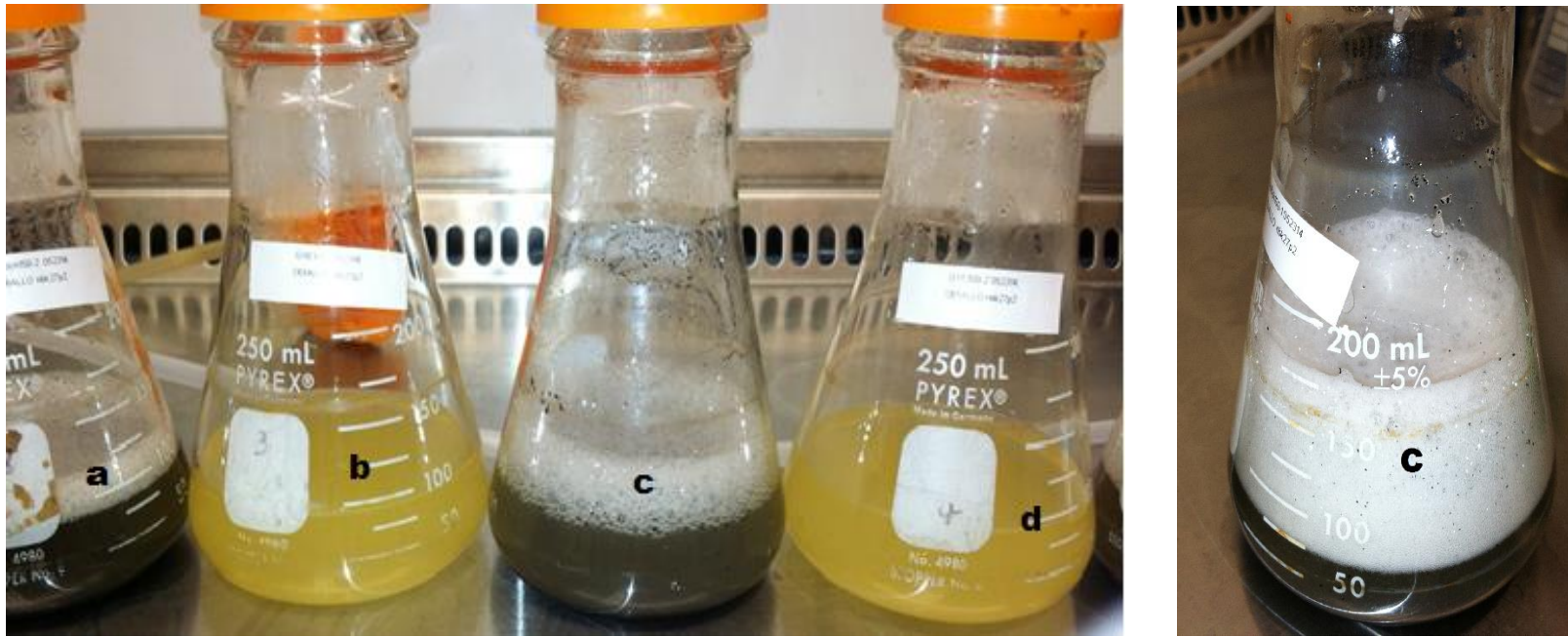
Figure 2.12. Fermentation of biochar (flasks a and c had bubbles) and control (flasks b and d had no bubbles) media at 9 h
