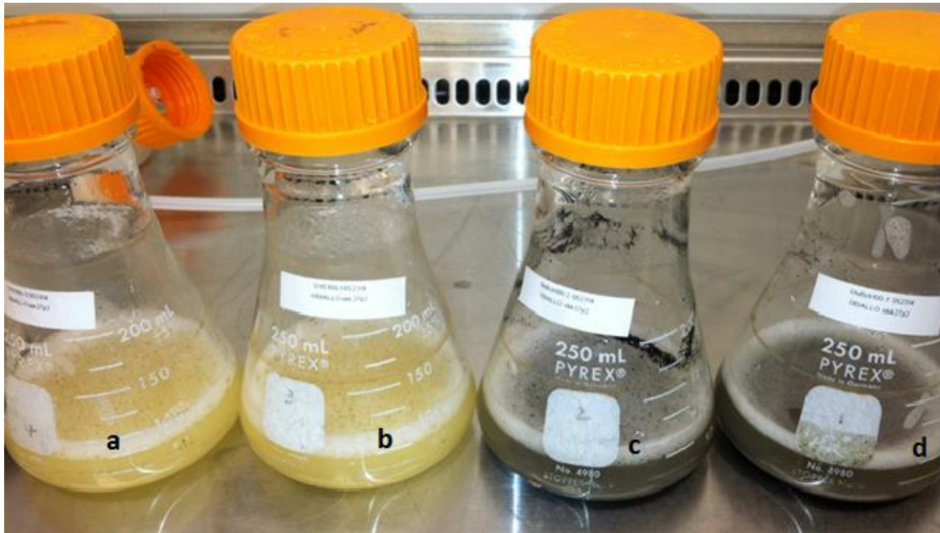
Figure 2.13. Fermentation of biochar (flasks c and d had bubbles) and control (flasks a and b had bubbles) media at 24 h
