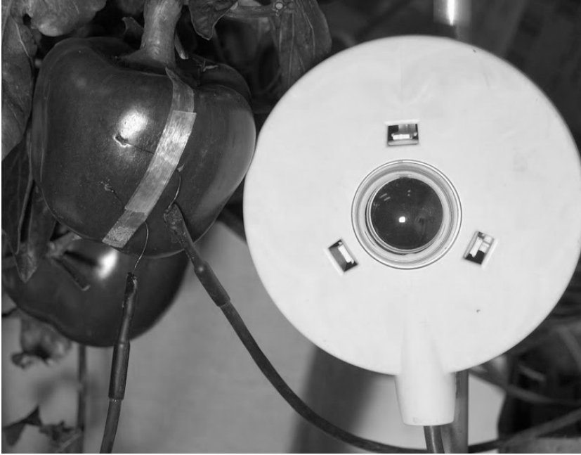
Figure 3.2. Thermistors and pyranometer located at approximately equally heights and distances from the light source.
