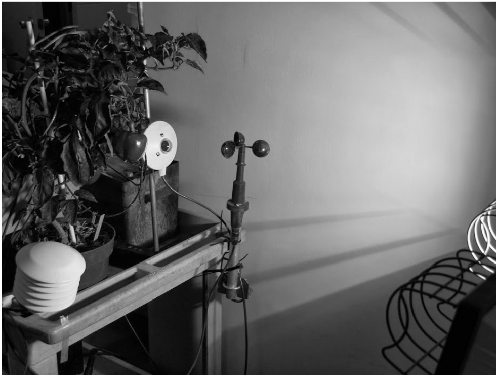
Figure 3.3. Light source, shielded thermocouple, cup anemometer, and pyranometer used during attached pepper fruit surface temperature measurement in a controlled environment.
