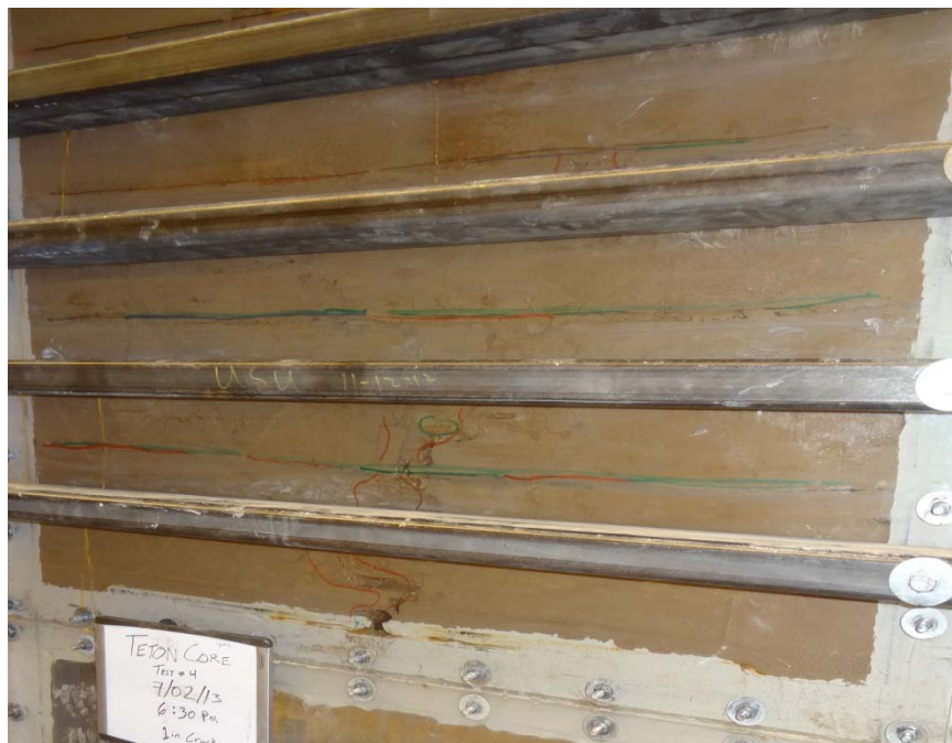
Figure 65. Teton Core test #3 35 days after start of test (visible channels marked in red)
