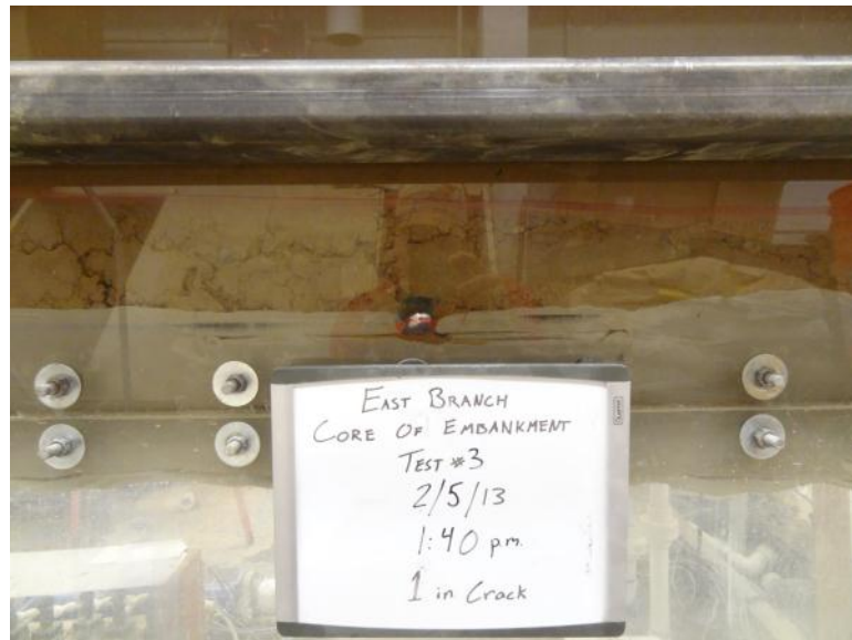
Figure A- 6. Test 3 on East Branch Core during Cycle 6 charge
