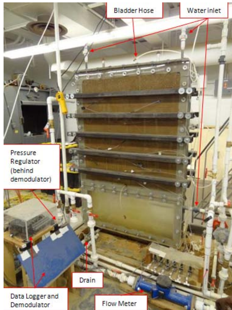
Figure 10. Photo of foundation void test cell
