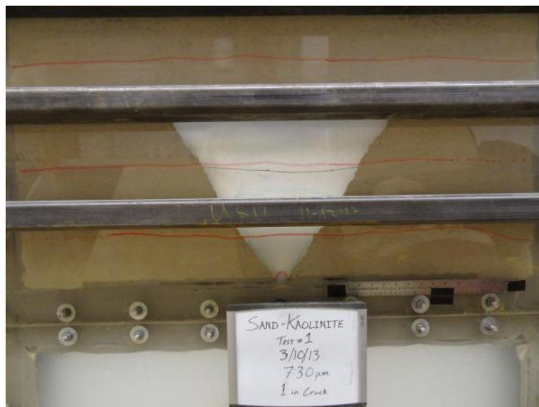
Figure A- 37. Test 1 on Sand with Clay during Cycle 6 discharge
