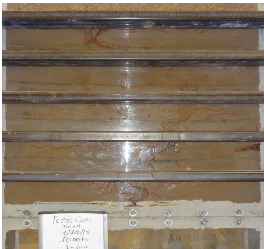
Figure 66. Teton Core test #3 43 days after start of test (visible channels marked in red)
