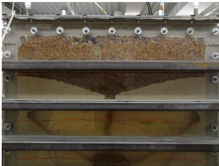
Figure A- 52. Test 1 on Sand with Clay during Cycle 11 discharge
