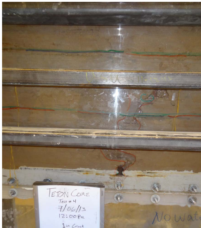
Figure A- 108. Test 3 on Teton Core with constant downward gradient
