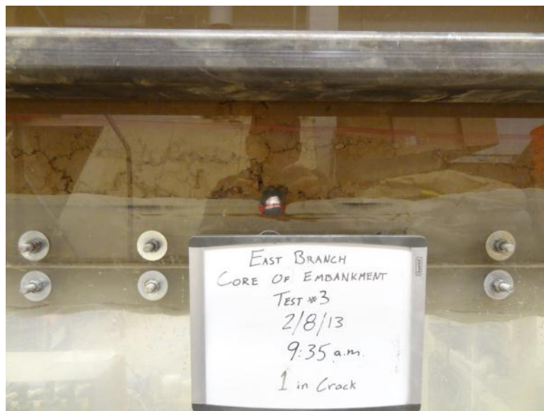
Figure A- 9. Test 3 on East Branch Core during Cycle 9 charge
