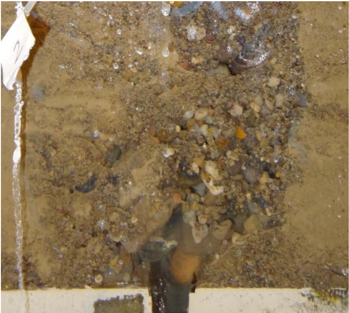
Figure 19. Natural soil filter around open void
