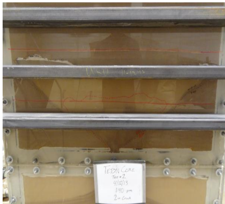
Figure 63. Teton Core test #2 at failure 2.5 hours after start of drainage of cycle 2
