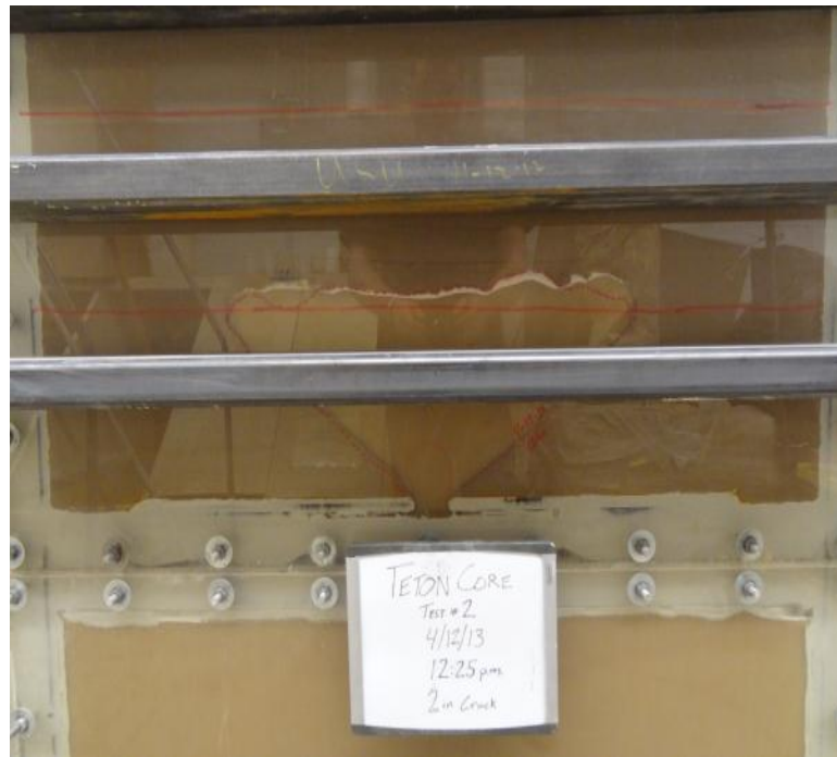
Figure 62. Teton Core test #2 one hour after start of drainage of cycle 2
