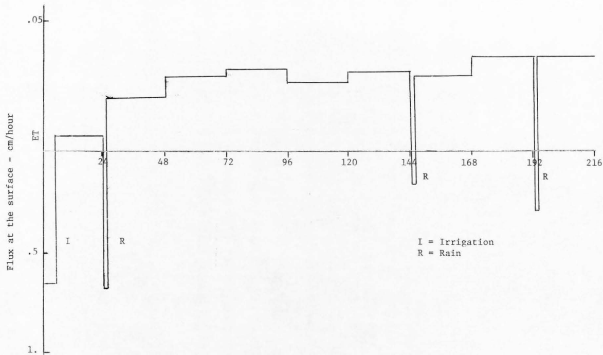
Figure 9. Water flux at the surface (evapotranspiration and precipitation cm/hr) vs time for oats in the 9-day interval in 1970.
