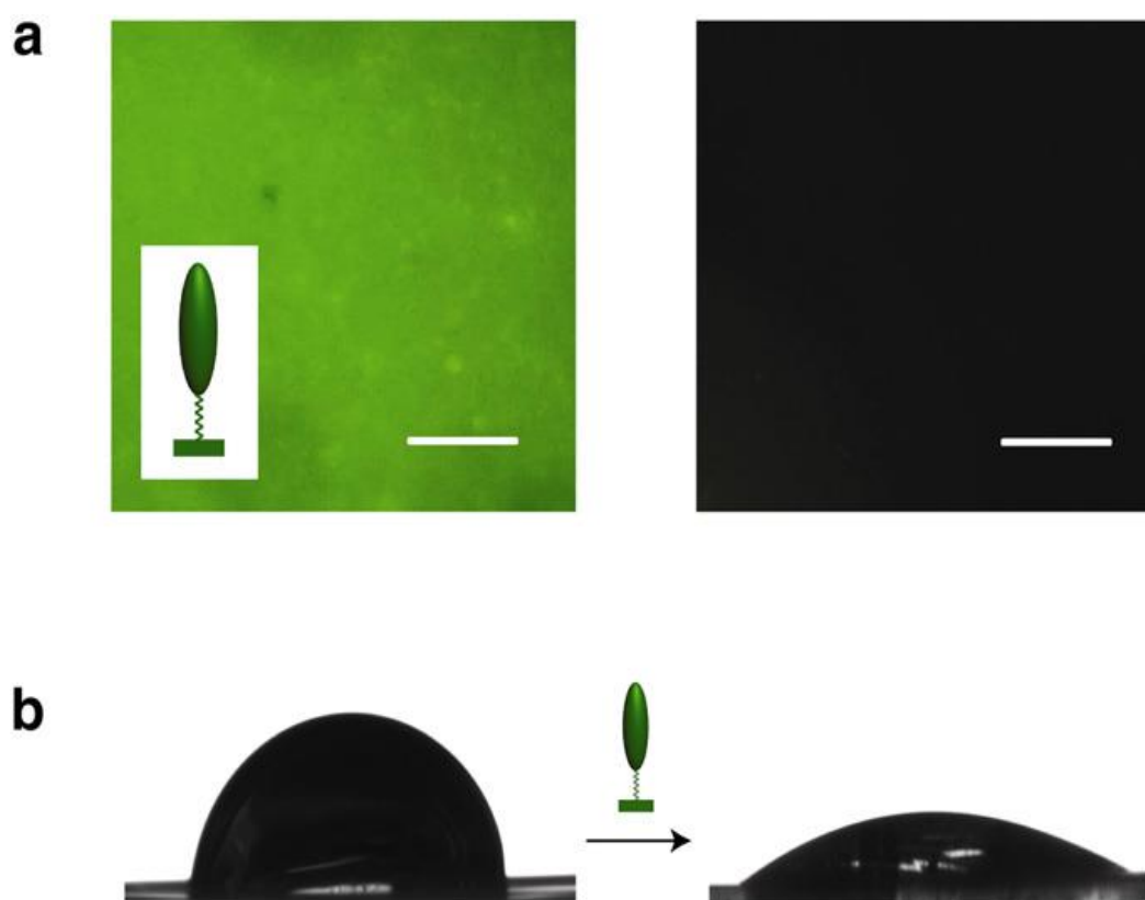
Fig.15. (a) Fluorescent characterization of the phage displayed peptide TLHPAAD on the plain epoxy surface and control with no phage displayed peptide, (b) Goniometer analysis of the phage displayed peptide on epoxy surface. Scale bar: 20 \mu\text{m} [26].
