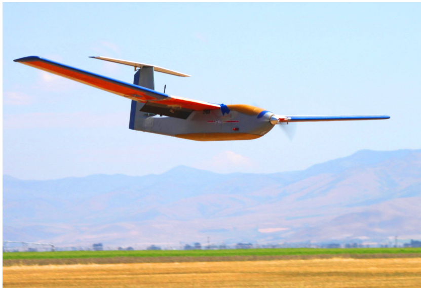
Fig. 6.1: Minion class personal remote sensing unmanned aerial vehicle
