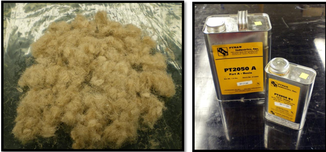
Figure 5: Chopped Fibers (left) and PT2050 Resin (right) Used for Composites
