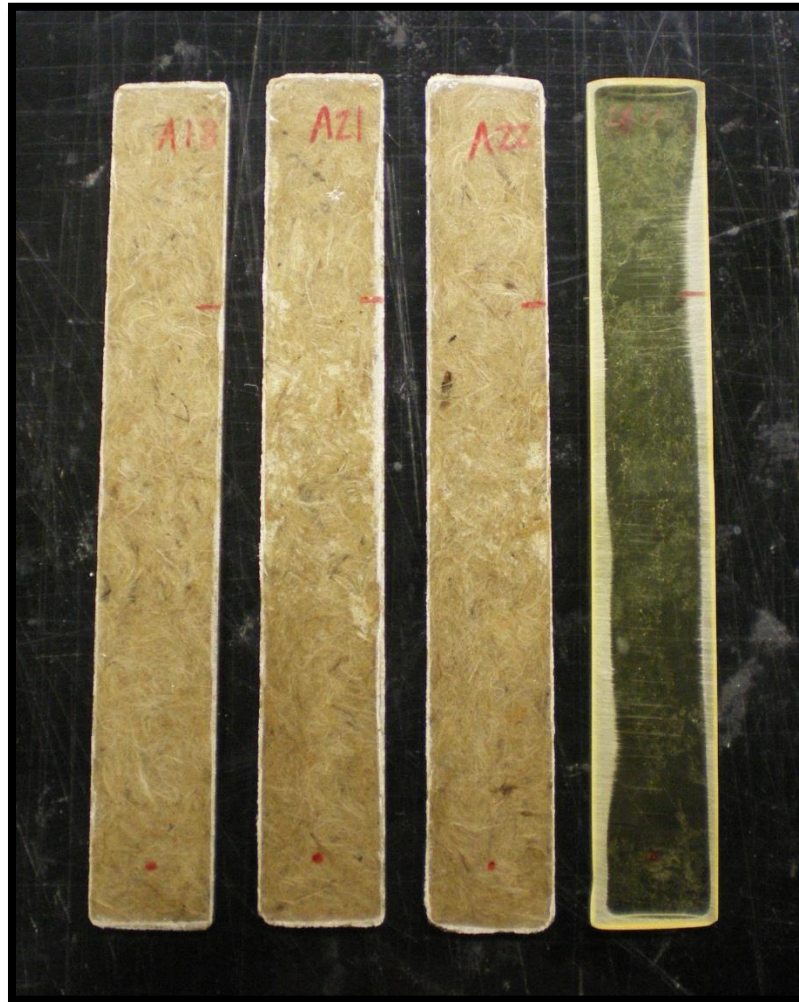
Figure 7: Cured Kenaf Fiber-Reinforced Composites and a Neat Epoxy Sample
